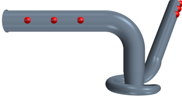
Figure 4.3: Pressure monitors location for c1 elb. The full outlet duct is not shown.
