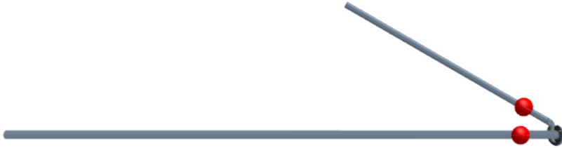
Figure 4.2: Numerical domain and location of the pressure probes for compressor c1 rsd.
