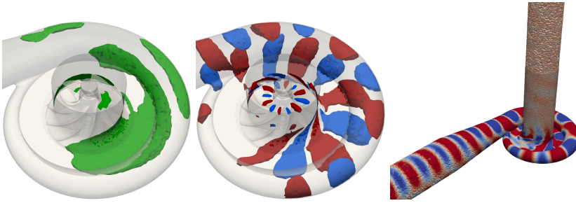
Figure 5.35: Maximum amplitude, modal shape and propagation of the BPF mode of c2 rsd nsg.
