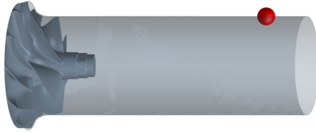
Figure 4.18: Numerical location of the pressure and FW-H probe at the inlet duct of c2 rsd geometry.
