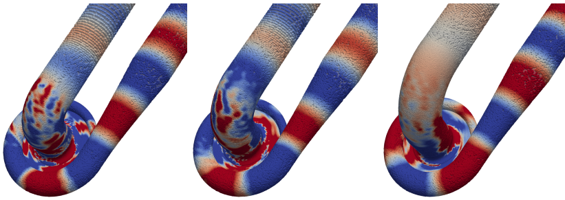
Figure 5.53: Propagation of the c2 nsg “whoosh modes” around 4000 Hz. From left to right: 0D75, e1D and e1D5. The inlet duct of the greater elbow radius (right figure) shows the lowest amplitude.
