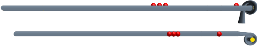
Figure 4.12: Numerical domain and location of the pressure probes for compressor c2 rsd.
