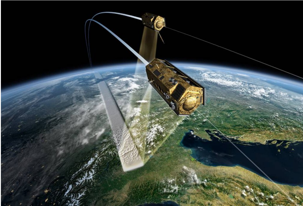
FIGURE 2.2: TanDEM-X and TerraSAR-X in formation flight. (Image credit: DLR)
