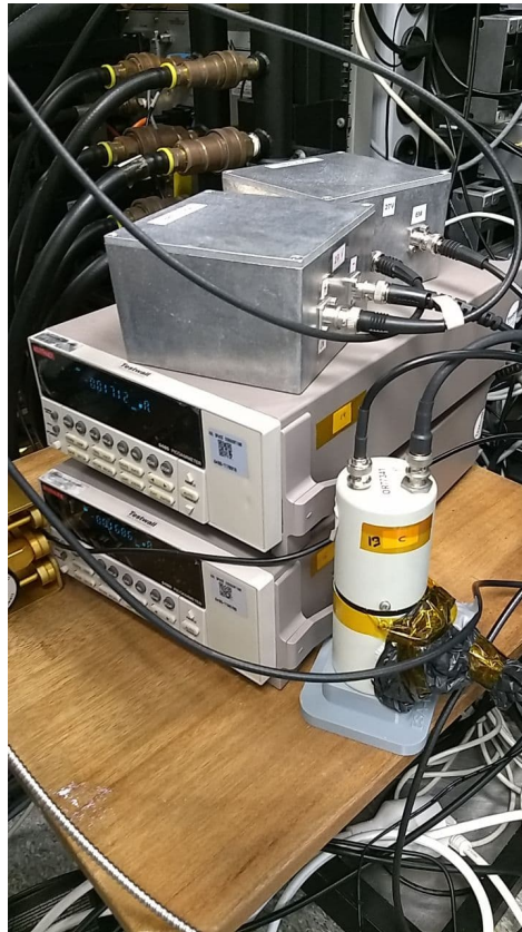
Figure 2.14: Two electrometer systems including their +30V bias boxes and a photomultiplier (right).
