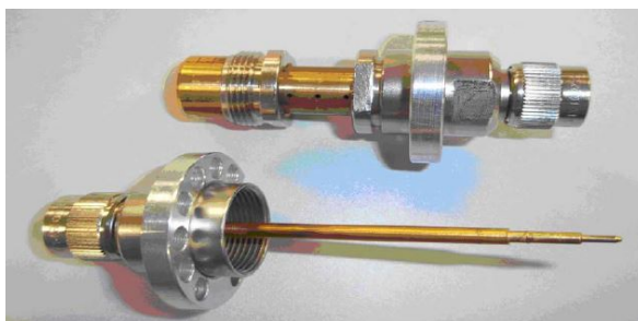
Figure 4.3: Example of a multipactor sample used for the multipactor analysis and experiments with digital modulated signals.
