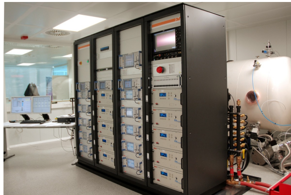
Figure 1.2: Ten channel and 2.4 kW CW Ku-band multicarrier facility. Photo credits: European High Power RF Space Laboratory, València, Spain.
