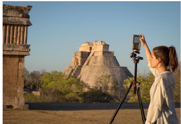
Figure 3. Laser scanning data capture at Uxmal, Mexico. (Photo R. Martínez 2018).
