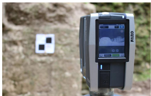
Figure 4. Data capture with a FARO Focus 3D S120 laser scanner, using bidimensional reference targets. (Project La Blanca 2015).
