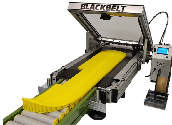
Figure 30. Wing printed on Blackbelt 3D printer.
