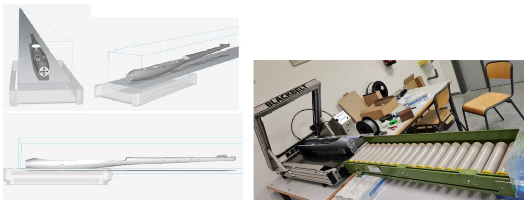
Figure 29. Fuselage set to be printed (left) and printed (right) with the Blackbelt printer.
