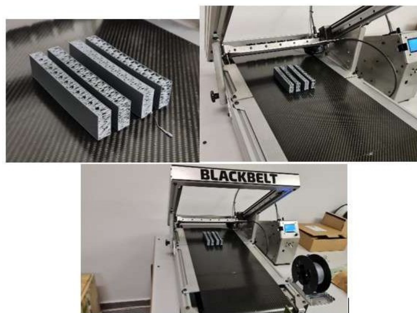
Figure 7. The Blackbelt 3D printer and the specimens printed.
