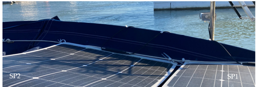
Figure 14. Shading shift from SP1 to SP2 at 16:00 h due to the antenna mast and sensors.
