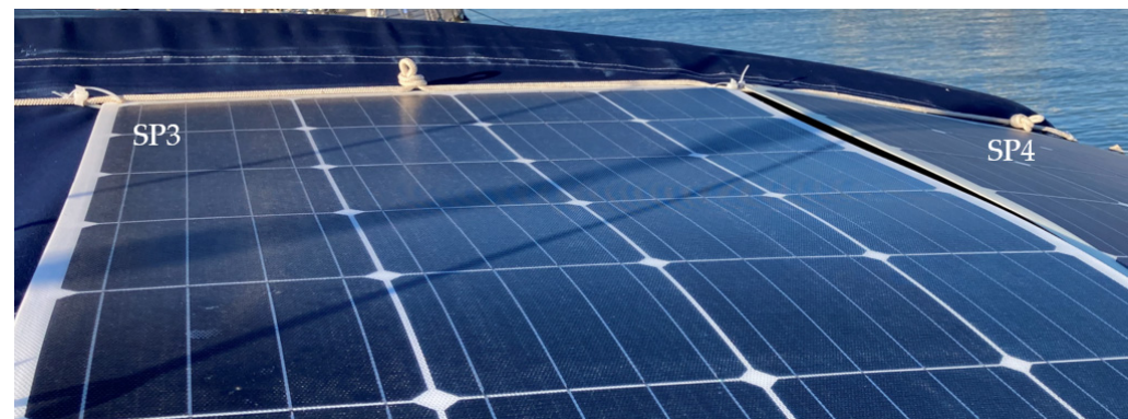
Figure 15. Shaded in SP3 and SP4 at 16:00 h in the position of the Sun at sunset from the Southwest.
