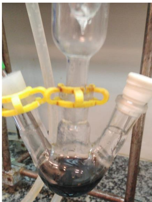
Figure 2-3: InP Quantum Dots doped with Vanadium.
