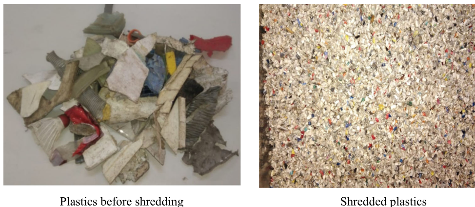
Fig. 3 Post-consumer plastics from solid urban waste (MSW) before and after being shredded
