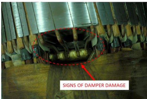
Fig. 3. Rotor of the CRSM and evidence of damper damage in CRSM1.
