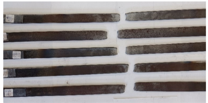
Figure 10 Specimens subjected to PFL tests. Failure shapes.
