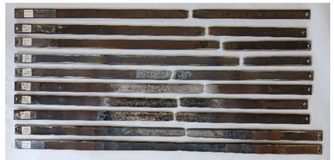
Figure 7 Failure shapes of specimens subjected to PFU tests. In the image, the upper specimen was heated to 100 °C, and, from up to down, to increasing temperatures at intervals of 100 °C (the lower was heated to 1000 °C).
