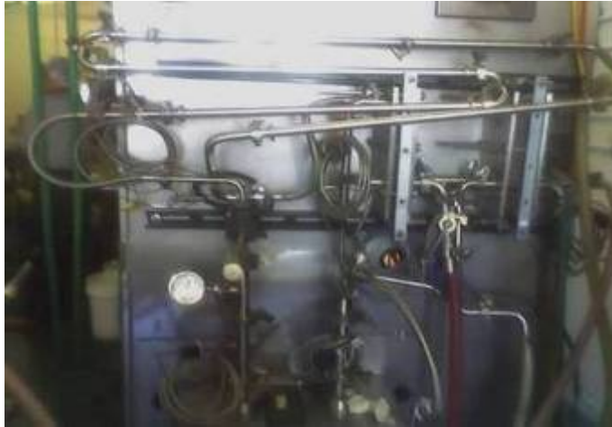
Figure 2.5.3-PEF industrial-scale equipment combined with a heat exchanger (Prof. H. Zhang).
