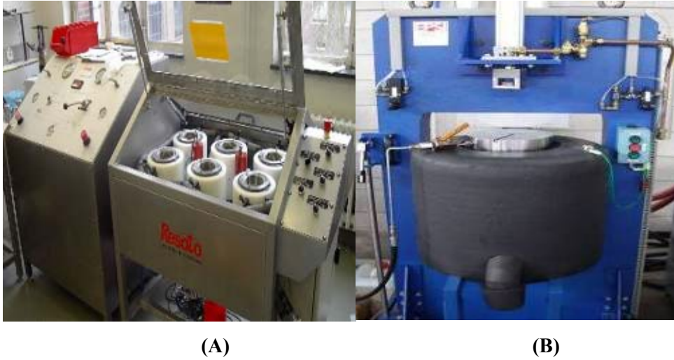
Figure 2.4.2: HHP lab-scale equipment: (A)-Laboratory of Food Process, Katholieke Universiteit Leuven, (Belgium), (B)-Instituto de Agroquímica y Tecnología de Alimentos, Valencia, (Spain).
