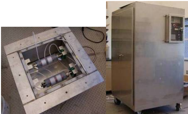
Figure 2.5.2- Treatment chambers-(A). PEF industrial-scale equipment-(B). Ohio State University, OH, (USA). (Prof. H. Zhang).
