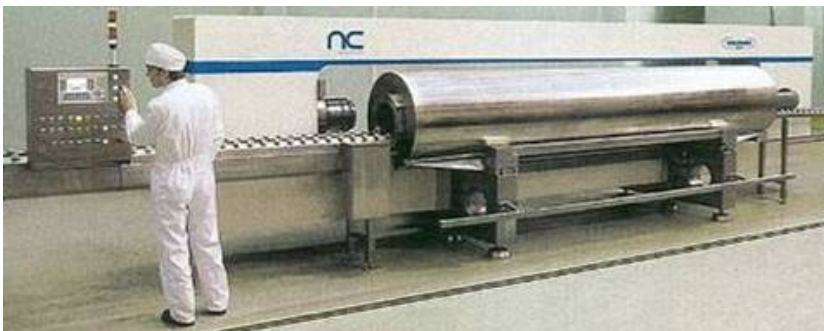
Figure 2.4.3: HHP industrial-scale equipment (Hyperbaric S.A., Burgos, Spain).
