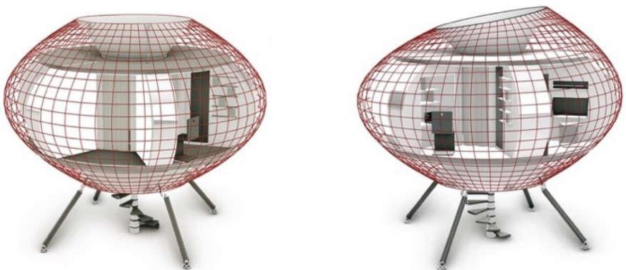
Figure 5. The result of associative parametric design and an instance of physics-based bending behavior simulation of the gridshell
