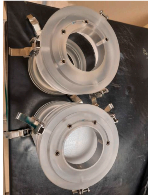
Fig. 3. The two upper part of the A10 of the LIAC used in this work. The top image shows the top view of both A10, with the designed filter embedded and the standard one. The bottom image shows the opposite view.
