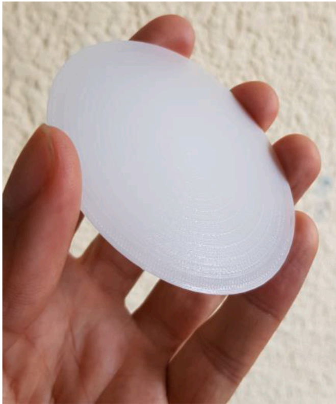
Fig. 2. Printed PLA (density of about 1.3 \text{ g cm}^{-3} ) designed filter which has been added to the A10 LIAC. The filter presents a conical shape with 1.3 mm height at the center.
