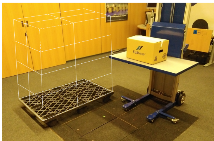
Figure 1. Picture of the laboratory configuration, showing the box over the destination table, and a schematic drawing in white of the initial configuration of the 16-box pallet.
