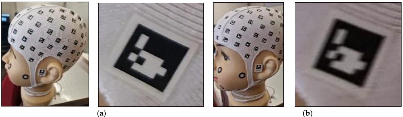
Figure 9. Comparison of input images: (a) Zoom in of an image obtained with the camera ( 4000 \times 3000 pix); (b) Zoom in of an image obtained with the video ( 1080 \times 1920 pix).
