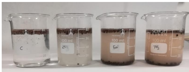
Figure S1. Appearance of 100 mL glass beakers with 80 mL of water and 50 seeds after ultrasonic treatments at powers of 0, 20, 50 and 100 W (from left to right) and a holding time of 60 s.
