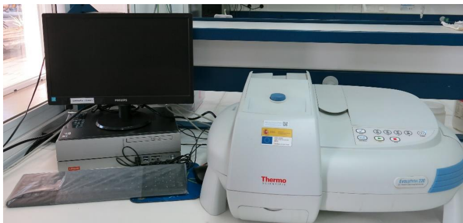
Figure III.4: UV-vis set up used in the TSA lab at the PSA with on the right the UV-visible light spectrophotometer and on the right the computer connected to it with the compatible software.
