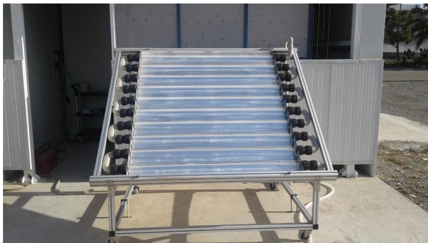
Figure III.15: Photo of the CPC reactor connected to the EO cell system as part of the EO pilot plant.
