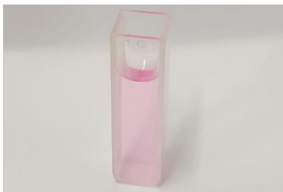
Figure III.5: Vial with a sample containing free available chlorine as indicated by the faint pink color.
