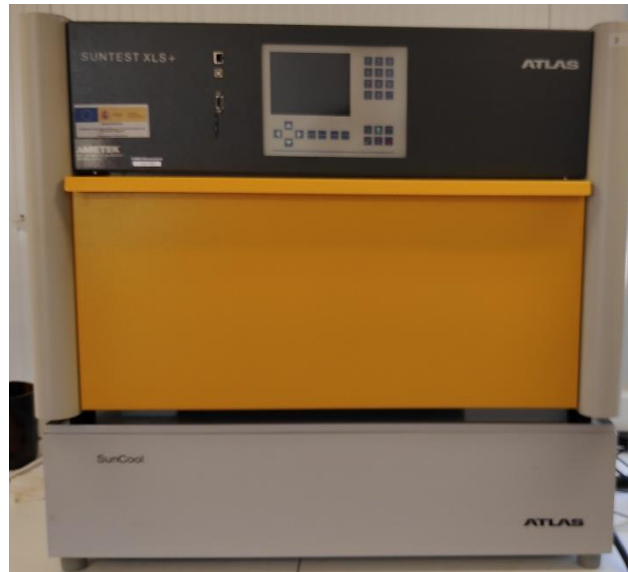
Figure III.18: The Atlas-SunTest XLS+ available at the PSA, equipped with a xenon lamp and a daylight filter.
