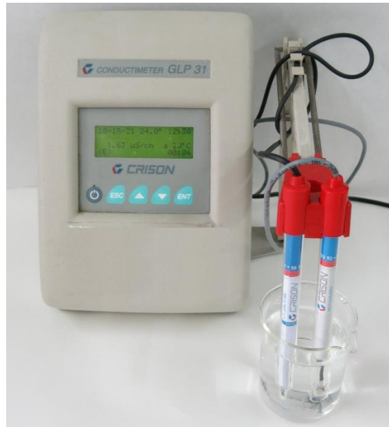
Figure III.1: Conductivity meter used in the TSA lab of the PSA.
