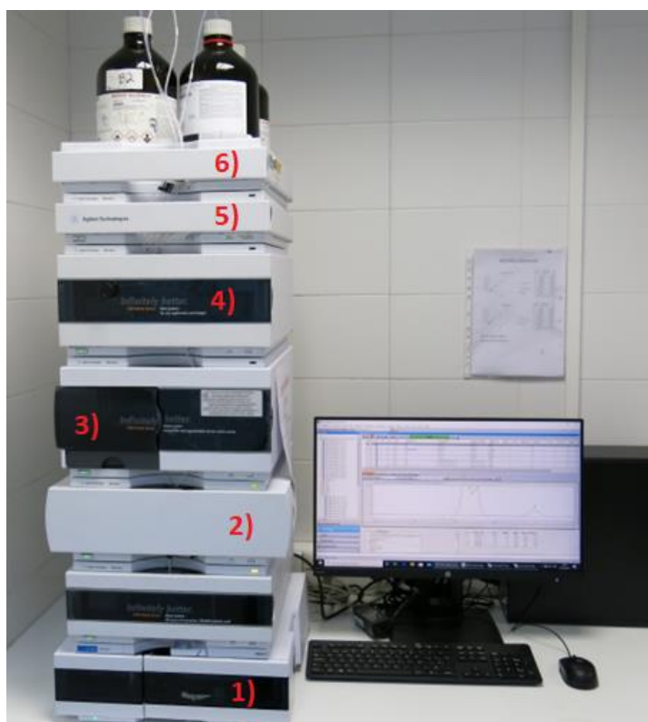
Figure III.8: UPLC used at the TSA lab of the PSA. With 1) Diode Array Detection (DAD), 2) column compartment with temperature control, 3) autosampler, 4) mobile phase pumps, 5) degasser, and 6) mobile phase tray.
