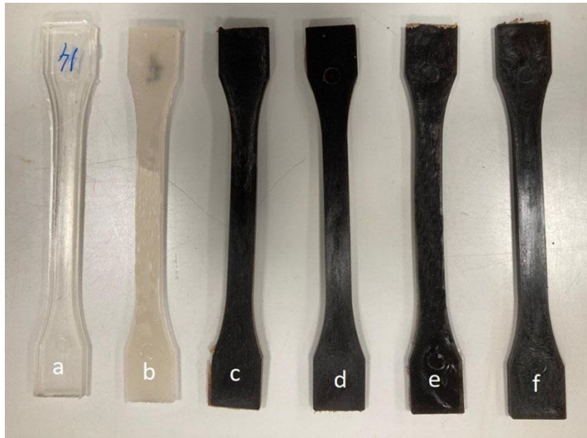
Figure III.2.2.6. Visual appeal of the samples: a) PLA; b) PLA+20TA; c) PLA+10TPF d) PLA+10TPF+22.5TA; e) PLA+20TPF+20TA and f) PLA+30TPF+17.5TA.
