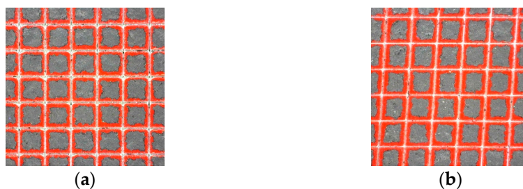
Figure 12. Lattice cut MTN_N2G_N x50 with Dino Lite® AD4113ZT: (a) initial adhesion; (b) effect of cold. Source: own authorship, 2023.
