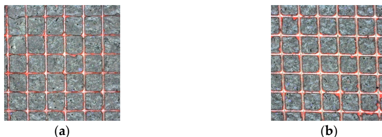
Figure 14. M_T x50 grating cut with Dino Lite® AD4113ZT: (a) initial adhesion; (b) effect of cold. Source: own authorship, 2023.
