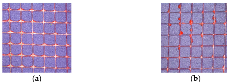
Figure 13. MTN_94_M x50 lattice cut with Dino Lite® AD4113ZT: (a) initial adhesion; (b) effect of cold. Source: Own authorship, 2023.
