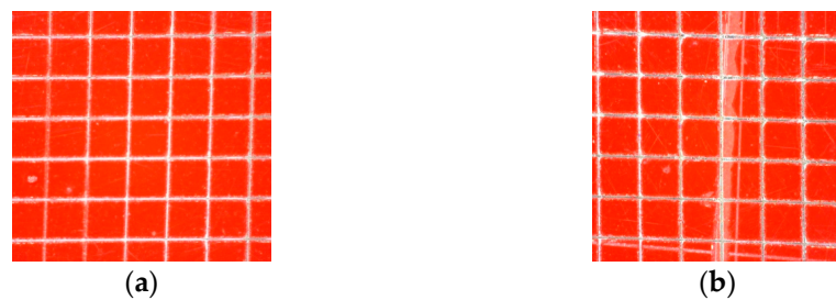
Figure 11. COA1 x50 grating cut with Dino Lite® AD4113ZT: (a) initial adhesion; (b) effect of cold. Source: own authorship, 2023.
