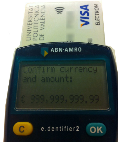
Figure 5.2: BECON_GetMode1Response - Challenge with maximal allowed amount sent to e.dentifier2 (Step 2 in the diagram of GetMode1Response, this picture was exactly taken before user pressed OK).
