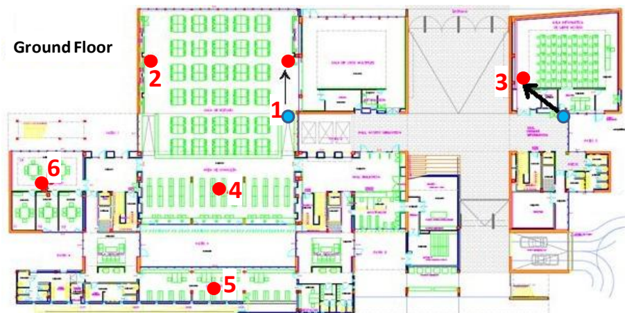
Figure 5.20. Relocation of APs on the ground floor
