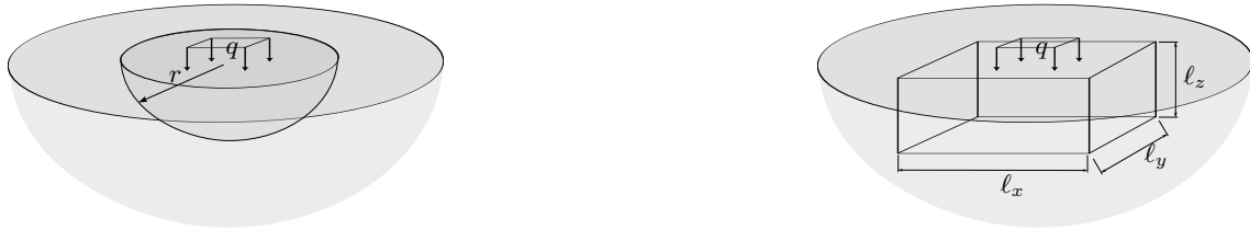
Figure 5: Infinite half space under constant area load q . (left) The computational domain is realized using a hemisphere. (right) The computational domain is realized using a cuboid.
