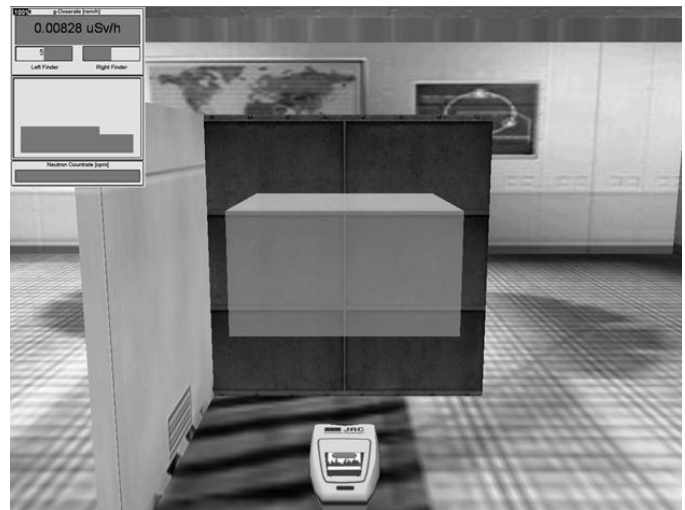
Fig. 10. User view of the application. A cubic source in the center. The walls around can be used to appreciate the result of the shielding (in real time) in the dose rate reading if the user walks behind them.
