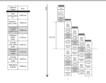
Fig. 9: Pipeline algorithm using different *streams* provided by the *concurrent copy and execution* property of GPU. On the left side, times spent by all stages of the algorithm
