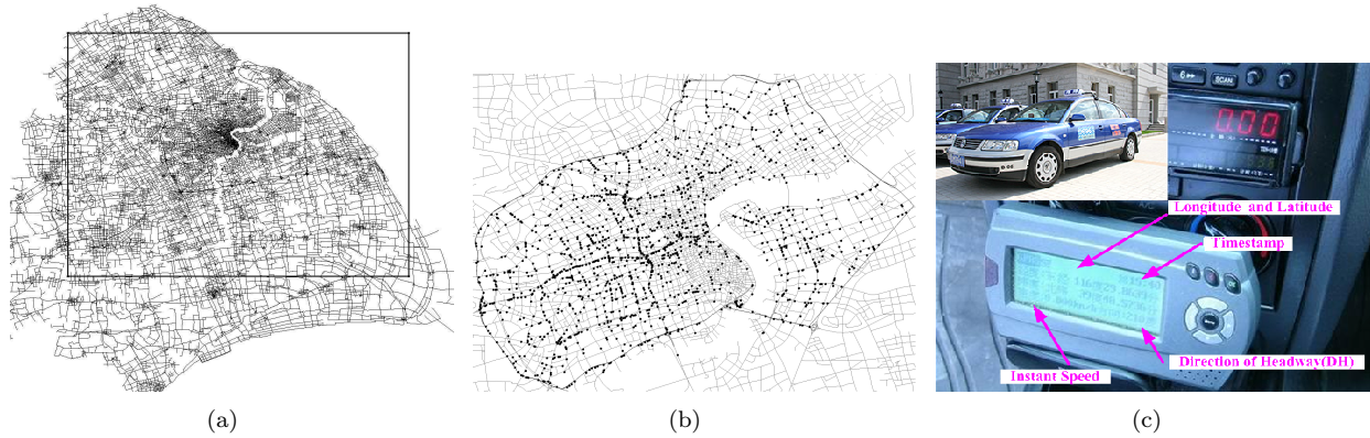
FIGURE 1. (a) The research area of Shanghai road map, where lines represent roads and black nodes refer to public buses or private cars, (b) A part of snapshots of Shanghai road map, (c) Vehicles are equipped with sensors.
