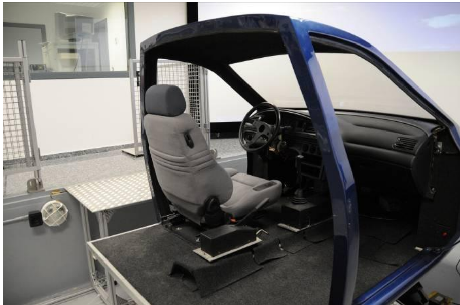
Fig. 2 Dynamic driving simulator
