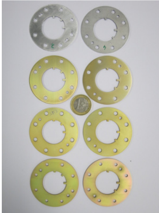
Figure 3.8 Insertion pieces of the original prototype and the three SM iterations (from top to bottom: original prototype, 1 st SM iteration, 2 nd SM iteration and 3 rd SM iteration).
