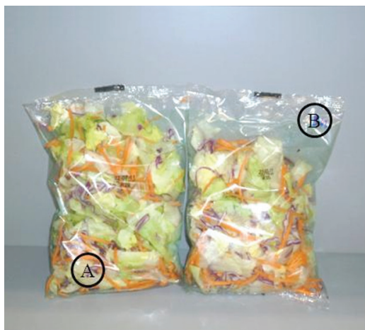
Figure 1. “Four season salad” bags in PP/EVOH films with oregano essential oil (A) and citral (B) in active modified atmosphere.
