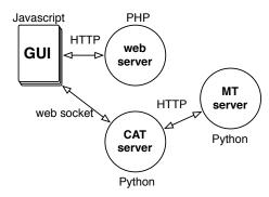
Figure 1 Components of the workbench
