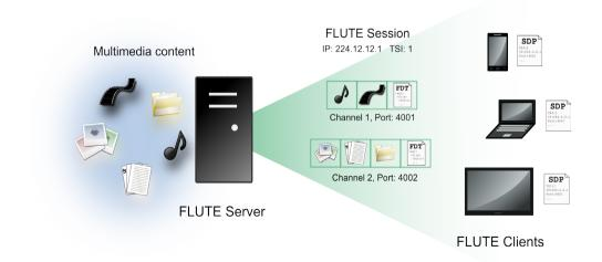
Fig. 2 File delivery using the FLUTE protocol
