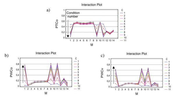
FIGURE 3: Interaction plots for diagnosis method × covariance structure: a)  $PTC_0$ , b)  $PWC_0$  c)  $PWC_v$ Arrows in the plots indicate the direction of increment of condition number of the correlation structures.
