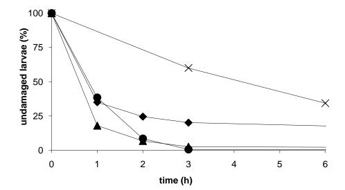
Figure 6: Pilot plant disinfection of water containg zebra mussel veligers by means of a circumneutral photo-Fenton process. Percentage of undamaged larvae (♠), and concentrations of hydrogen peroxide (♠) and iron (■) (both of them on right axis) are ploted vs. time. Undamaged larvae in the control experiment (solar irradiation) is also given (×). The initial concentration of veligers was between 50 and 100 larvae/ ml, (20 larvae/ml in the control experiment).
