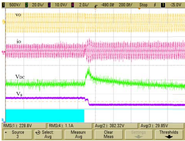
Fig. 21. Transient response for the transition from island mode to grid connected mode. v_O (first trace, 500V/div). i_O (second trace, 2A/div). V_{DC} (third trace, 20V/div). V_g (fourth trace, 10V/div). Reconnection signal (fifth trace). Time scale=200ms/div.
