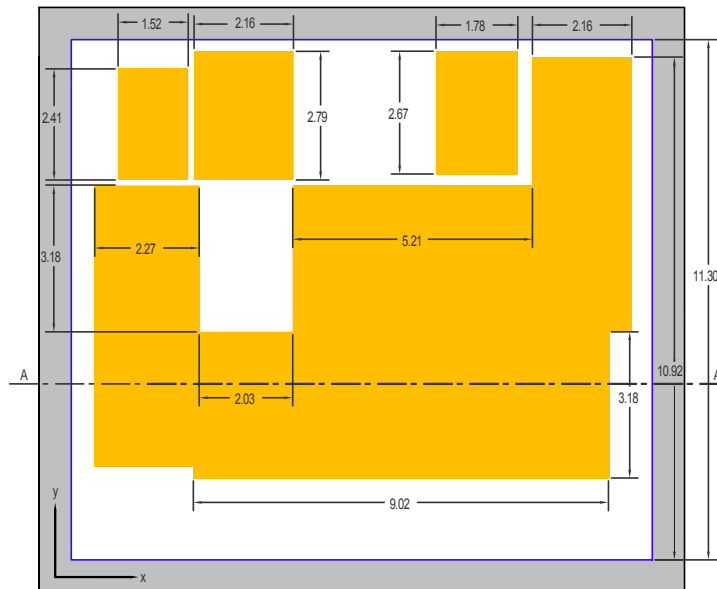
Fig. 2. Top View of Maine Yankee spent fuel storage pool.
