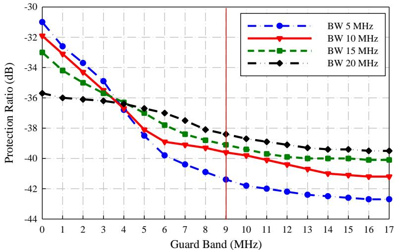
Fig. 3. Protection ratios for DTT interfered by LTE-UL for different LTE BW.
