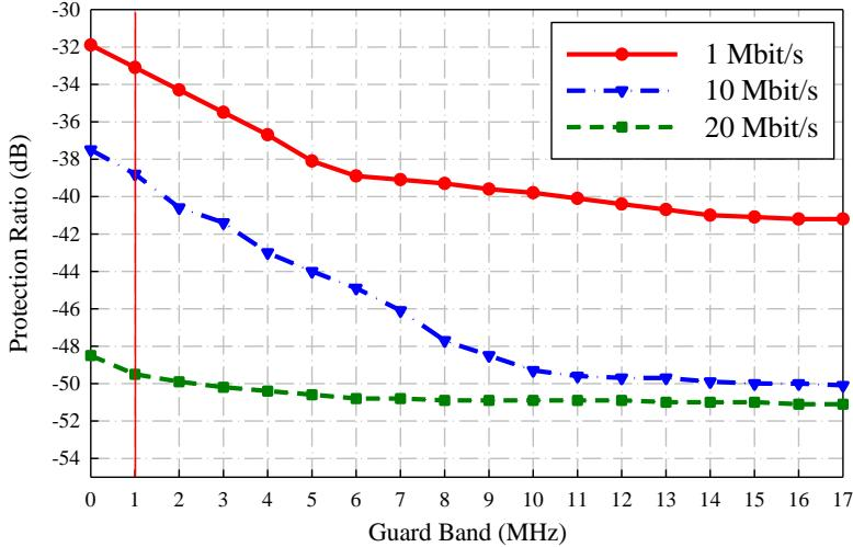
Fig. 2. Protection ratios for DTT interfered by LTE-UL with a bandwidth of 10 MHz, for different traffic loadings.
