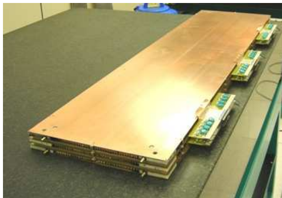
Figure 6.54: A M1R4 chamber completely assembled before the installation of the Faraday cage. The three honeycomb panels are visible. On the corners of the panels there are plastic inserts with internal channels for gas circulation. The gas nipples are inserted in the top and bottom panels. Decoupling HV capacitors, resistors and connectors for the FE boards are mounted on the printed circuit boards on the right.
