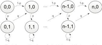
Fig. 4. State transition diagram for the Markov model in the transmission of n packets.
