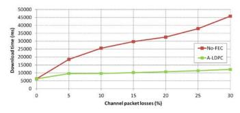
Fig. 6. Comparison between Adaptive LDPC and Compact No-Code with 3000 packet file size, 1 block, b=5 Mbps and t\_fd=3 s.
