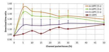
Fig. 10. Download time ratio with rateless codes with 3000 packet file size, 1 block and b=5 Mbps.
