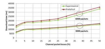
Fig. 7. Comparison between analytical and experimental results in a file size evaluation with 1 block, b=5 Mbps and t\_fd=3 s.
