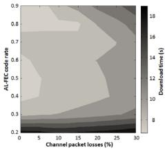
Fig. 5. Download time evaluation with LDPC Staircase codes with 3000 packet file size, 1 block and b=5 Mbps.
