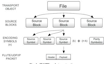
Fig. 1. FLUTE packet construction.
