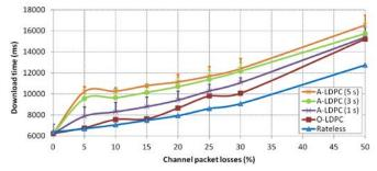
Fig. 9. Feedback time evaluation with 3000 packet file size, 1 block and b=5 Mbps.
