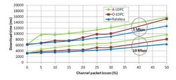
Fig. 11. Transmission rate evaluation with 3000 packet file size, 1 block and  $t_fd=3$  s.
