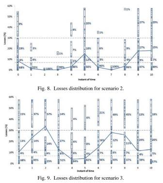
In the second scenario, the distribution of losses is different, existing time intervals when clients get closer to the server and others when clients move further away from it, as Fig. 8 shows. In addition, in the third scenario (Fig. 9) the losses are, in general, rather higher.
