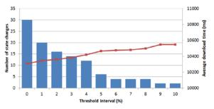
Fig. 22. Number of state changes and average download time depending on the threshold interval in scenario 5 for  $N_h$ =1/3,  $N_m$ =2/3.
