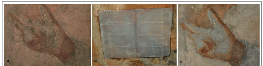
Figure 3. View of the particular wall painting area before (a), during treatment with agar as a carrier (b), and after (c) bacterial treatment. Animal glue rests can be seen in the left image (a) as black spots, and their correct removal in the right image (c).
