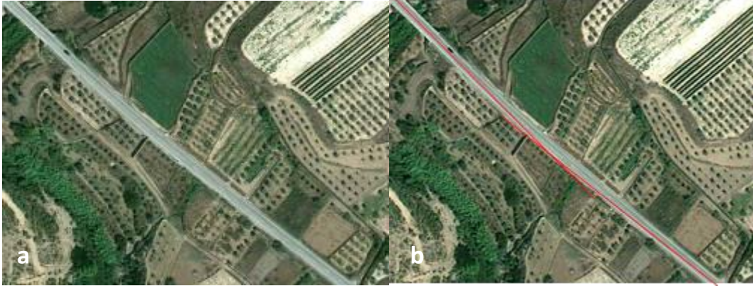
Figure 8 Example of a curve with a low deflection angle. This curve is hardly detected by other methodologies, but easily found with the one presented in this paper.
