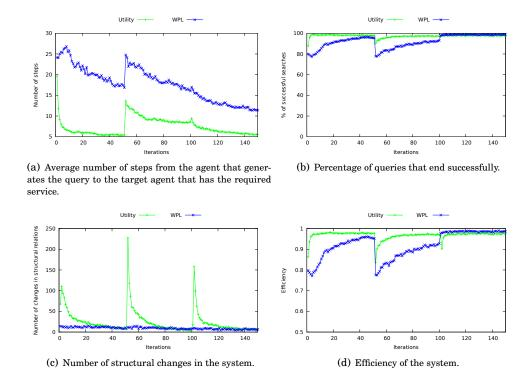
Fig. 7. Evolution over time of system measures considering dynamic changes in the service demand and different adaptation mechanisms: Utility and WPL.
