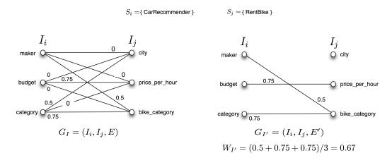
Fig. 2. (Left) Full connected weighted bipartite graph  $G_I$ , and (Right) resulting maximum weighted matching relaxed bipartite graph  $G_I'$ .
