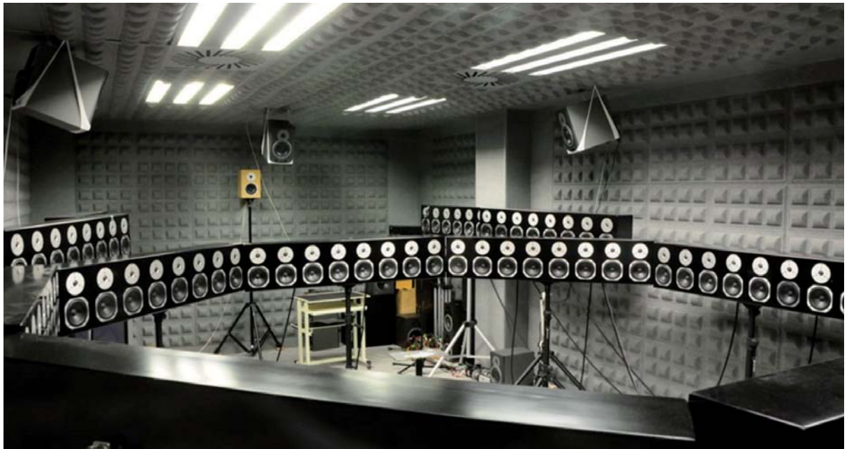
■ Figure 4. Wave-Field Synthesis set-up, where the octagon with the 64 loudspeakers can be appreciated and also the reference loudspeakers at the back in brown color.
