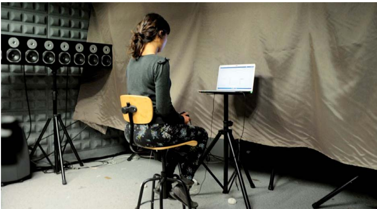
■ Figure 7. Participant seated in the listening position ready to start the test. The laptop computer with the GUI, the joystick and the acoustic curtain can be appreciated.
