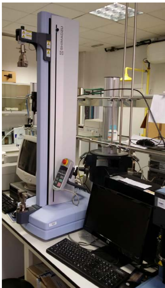
Figure 3.20. Picture of a Hounsfield H10KM Universal Testing Dynamometer.
