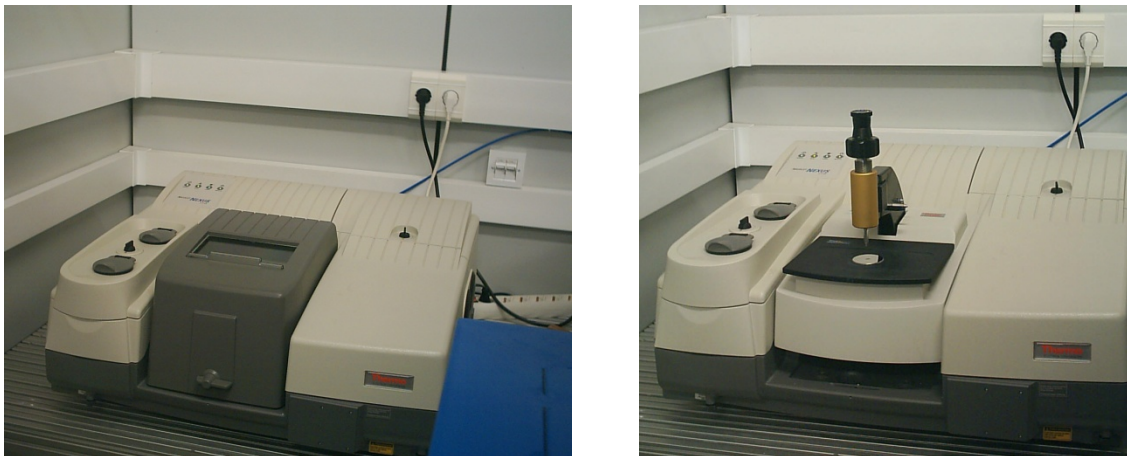
Figure 3.7. Pictures of Nicolet Nexus FTIR spectrometer.
