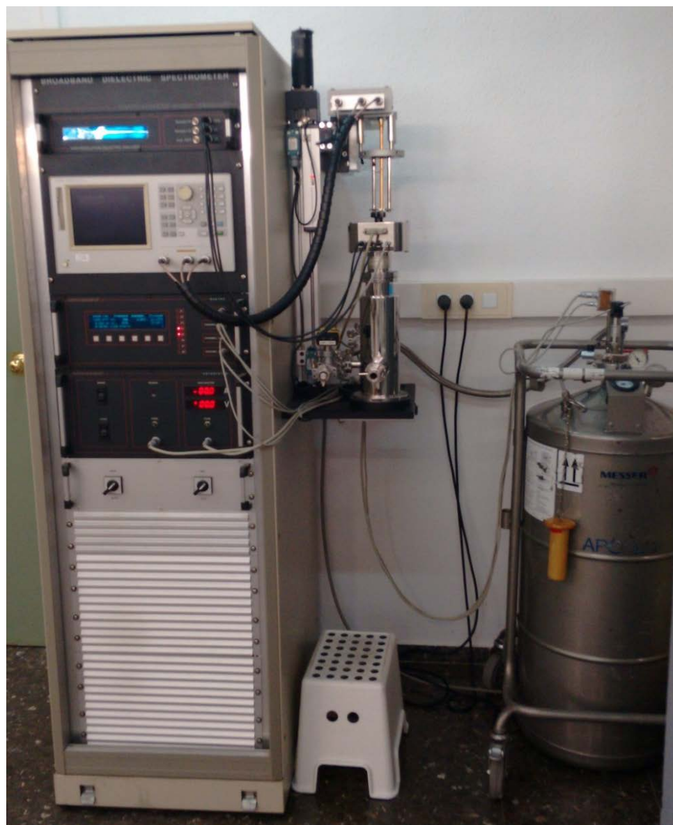
Figure 3.17. Picture of the Novocontrol Concept 80 instrument and the liquid nitrogen dewar.
