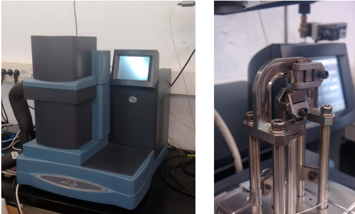
Figure 3.23. Picture of the TA Instruments DMA Q800 (left) and the tension mode clamp used in the measurements (right).
