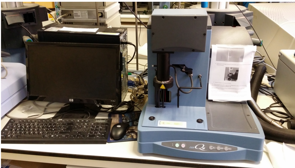
Figure 3.8. Picture of the TA Instruments Q50 TGA analyzer.
