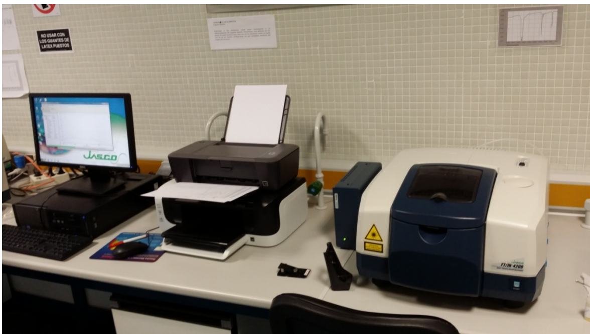
Figure 3.6. Picture of the JASCO FT/IR-4100 spectrometer.
