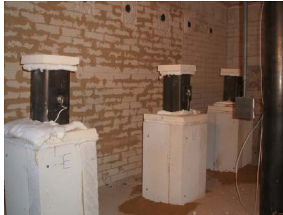
Fig. 4. Location of test specimens in furnace.
