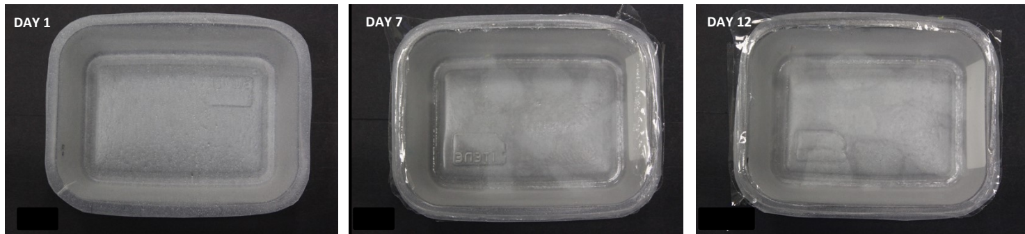
Figure 4.71. Visual aspect of the active trays previously packed with orange at 4 °C for 7 days followed by 5 days at 8 °C
