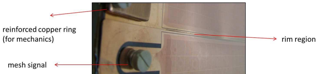
Figure 4. Close up of the ‘rim technique’ used for reducing charge loss in multi-wafer Micromegas assemblies when aimed at large area coverage.
