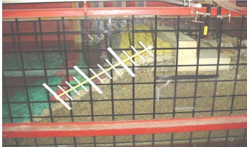
Figure 3-2. Double-layer Cubipod armor with R_c=20.33 cm.
