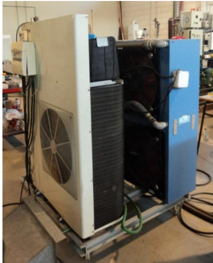
a) Heat removal circuit
