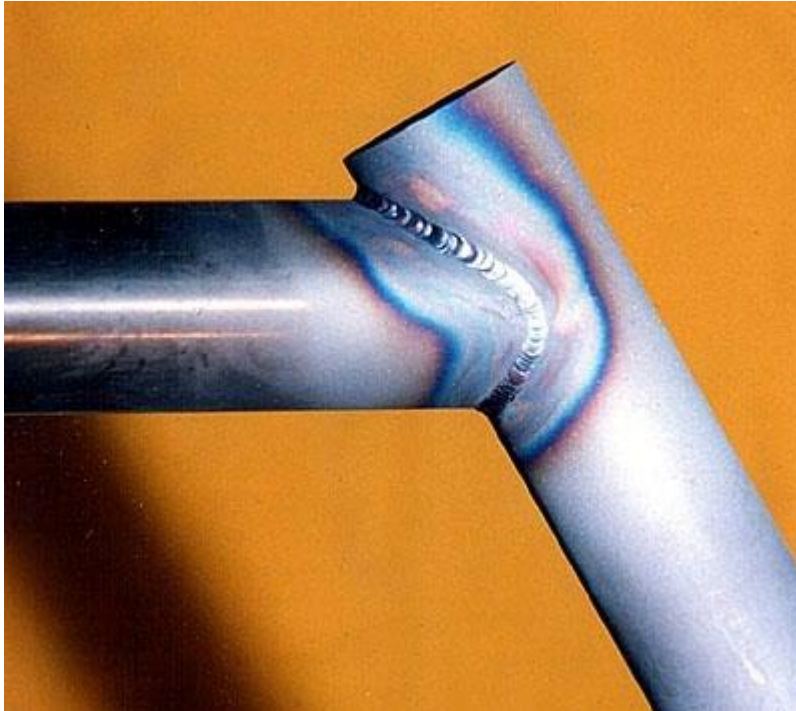
Figure 12. Welded steel tube frame joint. Retrieved from http://www.bikerumor.com/2015/01/16/how-to-build-a-nahbs-bike-part-4-melting-tubes-together/
