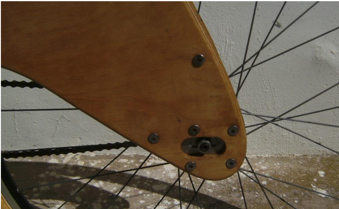
Figure 184. 3mm Original Steel Plate Dropouts Contoured to fit Frame. Taylor, Nicholas.
