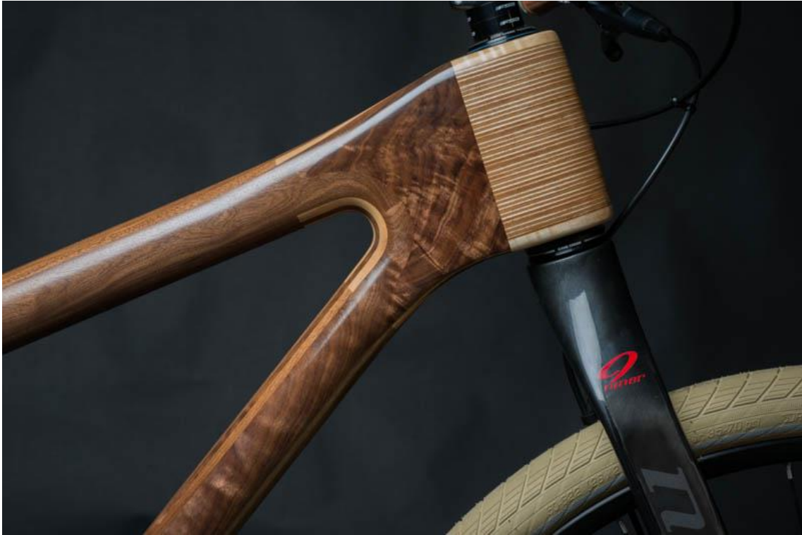
Figure 107. Laminated Wood Head Tube Detail – AnalogOne. Retrieved from http://www.blessthisstuff.com/stuff/vehicles/cycles/analogone-one-bicycle-by-grainworks/
