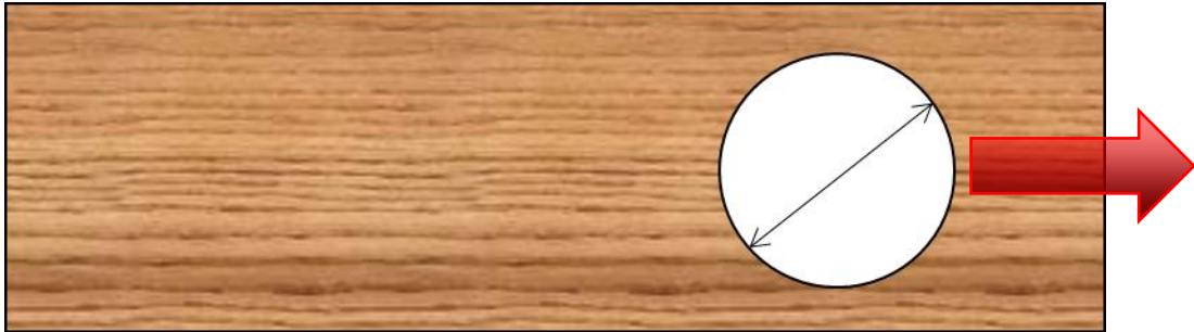
Figure 128. Top View of Wooden Core – Grain Direction and Steerer Tube Position – Taylor, Nicholas.
