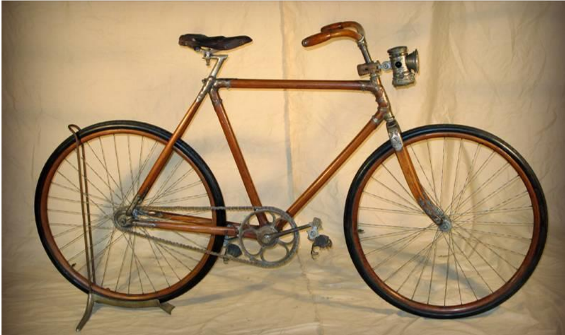
Figure 93. Hickory Diamond framed Bicycle circa 1910. Retrieved from http://www.sterba-bike.cz/produkt/old-hickory-lady-wood-bicycle-1898?lang=EN
