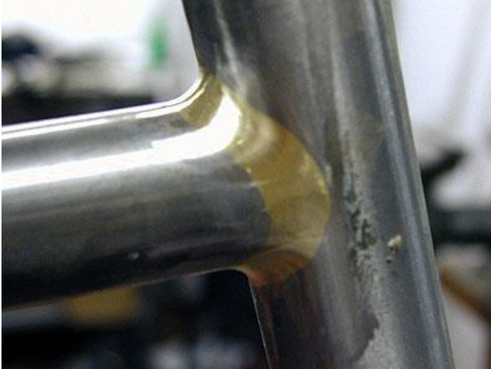
Figure 11. Fillet brazed frame joint. Retrieved from http://www.ecovelo.info/2010/01/23/fillet-brazed-frames/
