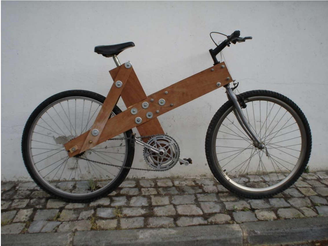
Figure 147. Xylon #1 Full Size Prototype During Initial Trials –Taylor Nicholas.
