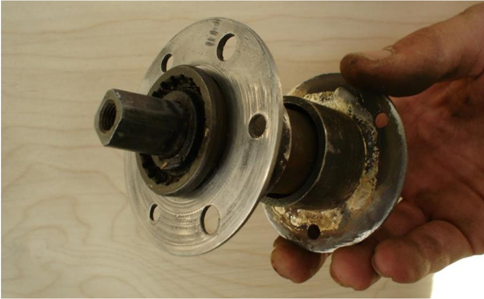
Figure 194. Two part flanged bottom bracket fabricated and brazed. Taylor, Nicholas. 2005
