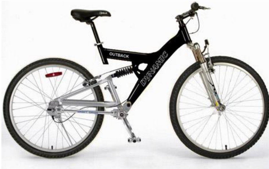
Figure 29. Unusual shaft drive Dynamic Outback mountain bicycle. Retrieved from http://www.dynamicbicycles.com/
