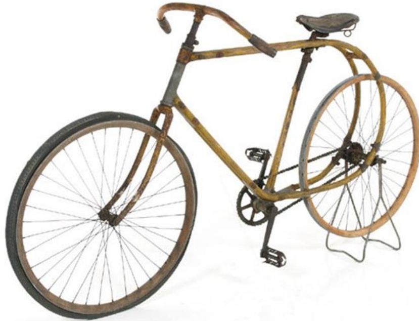
Figure 84. 'SOUPLETTTE' Bicycle with bent wood frame France circa 1898. Retrieved from http://www.sterba-bike.cz/album/659/category/the-gallery?lang=EN
