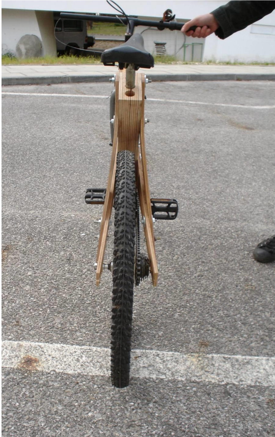
Figure 143. Xylon #1 Initial Trials – Rear View Showing Chain Line –Taylor, Nicholas.
