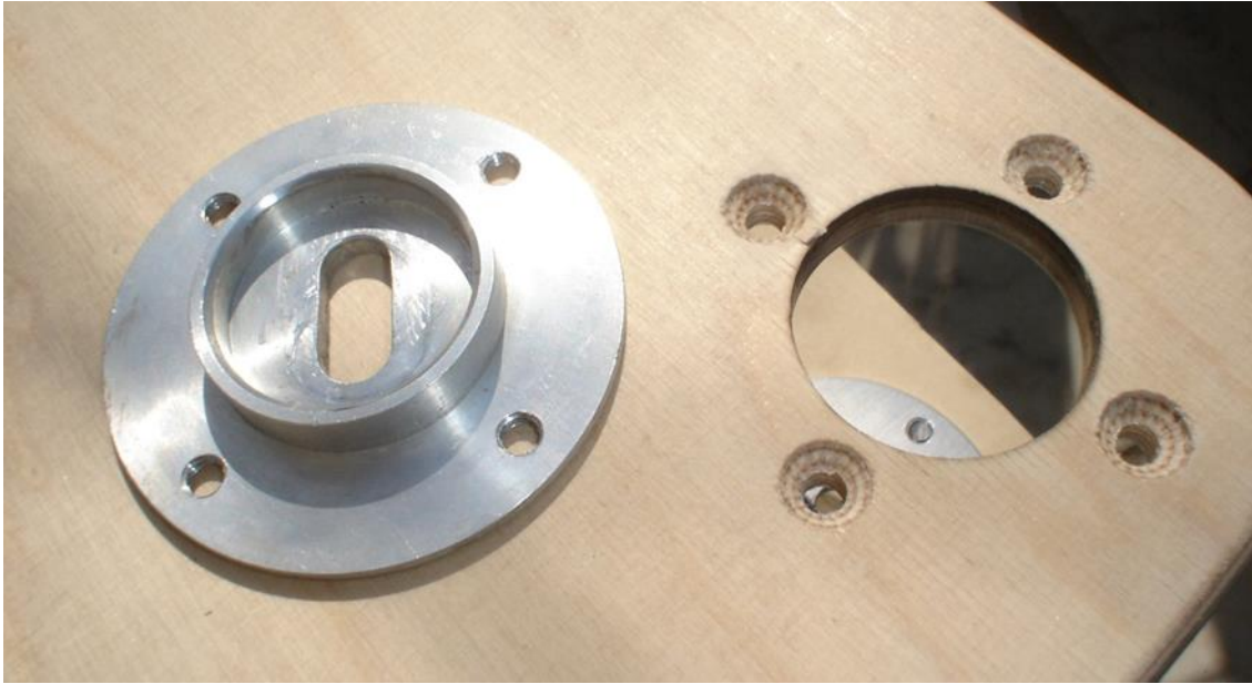
Figure 187. Xylon Turned Aluminium Dropout Prototype #1 Fitting to Frame. Taylor, Nicholas. 2007
