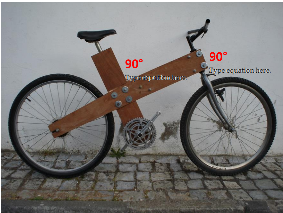
Figure 141. Xylon #1 Initial Trials – Full Size Cross-Frame Construction –Taylor, Nicholas.
