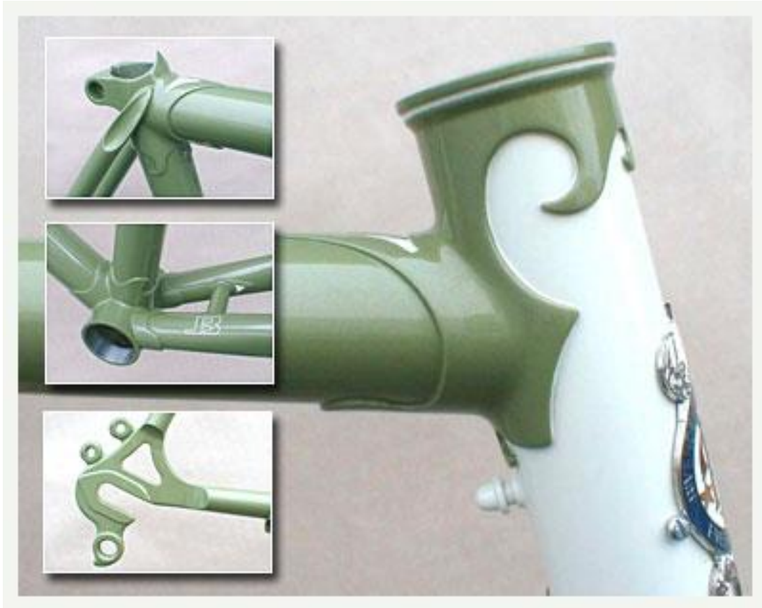
Figure 18. Contemporary lugged steel frame Rivendale Bicycles. Retrieved from http://www.rivbike.com/
