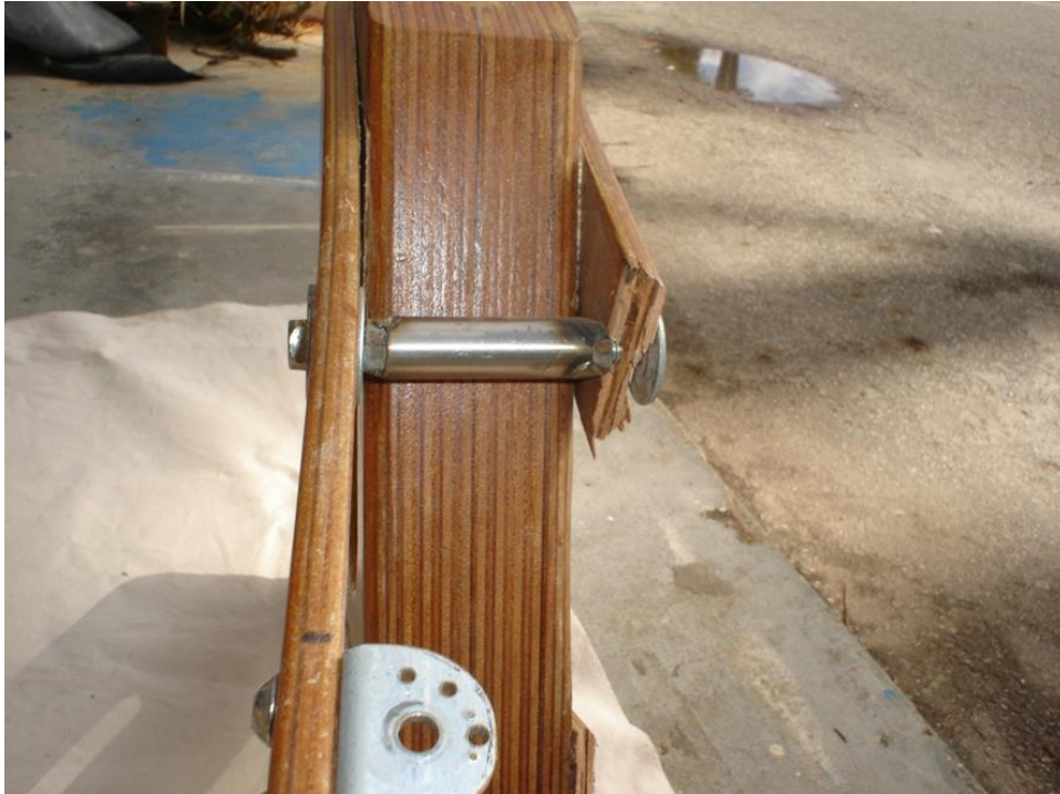
Figure 152. Detail of Failure on Xylon #1 Prototype at Rear Bracing Tie –Taylor, Nicholas. 2006
