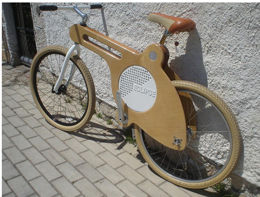
Figure 168. Mock-up of E-bike Based on the Xylon Eclipse Frame – Taylor, Nicholas. 2013
