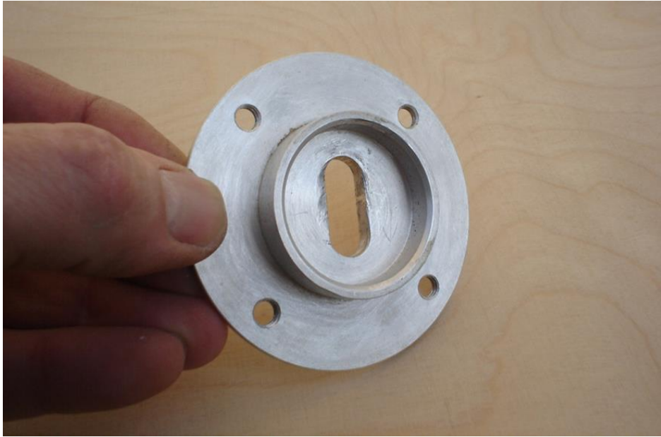
Figure 185. Xylon Turned Aluminium Dropout Prototype #1. Taylor, Nicholas. 2007
