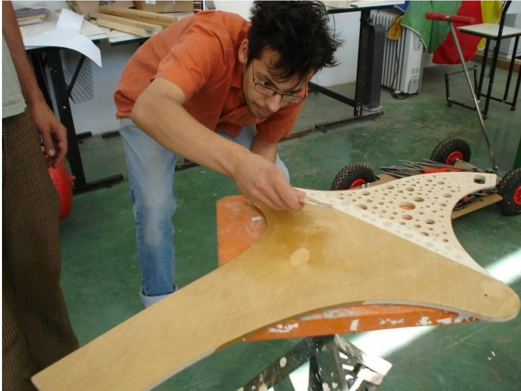
Figure 173. Sergio Cordeiro preparing Cell side panel prior to gluing and clamping. Taylor, Nicholas. 2005
