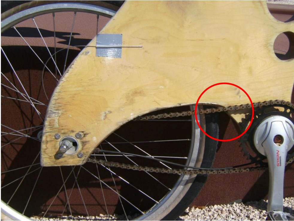
Figure 180. Xylon Hybrid showing Discolouration, Flaking Lacquer, and evidence of Chain Slap –Taylor, Nicholas. 2015
