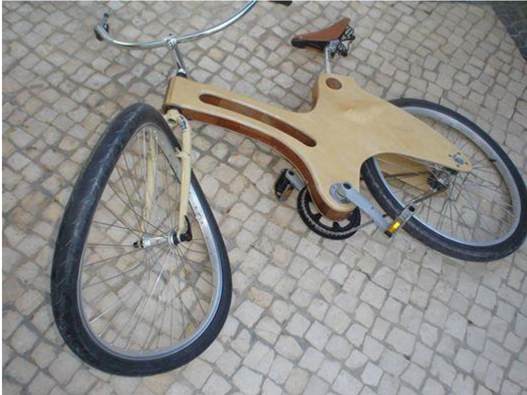
Figure 208. Xylon Classic after head on collision with a “conventional” steel framed bicycle.
