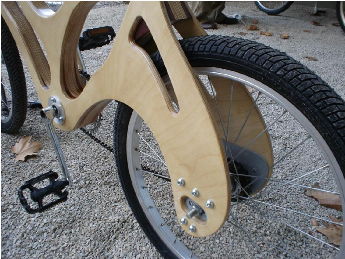
Figure 183. Xylon Synergy showing Slotted Frame and 3mm Steel Plate dropouts. Taylor, Nicholas. 2005
