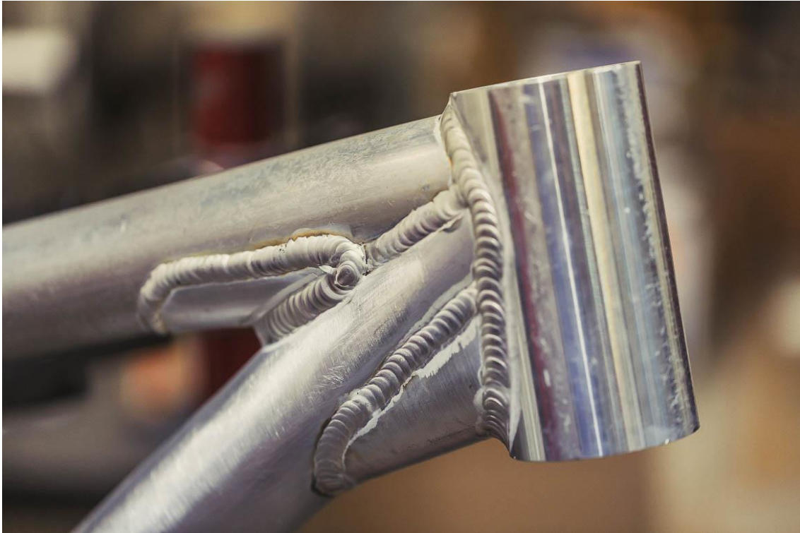
Figure 21. Welded aluminium frame head tube with reinforcement fillets. Guerrilla Gravity Bikes USA. Retrieved from http://ridegg.com/
