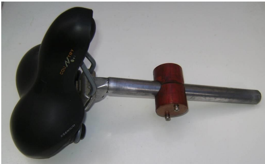
Figure 203. Xylon Wooden Seat post Clamp Prototype #2 Shown in Position on Seat-post. Taylor, Nicholas. 2010
