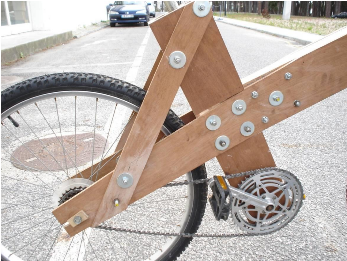
Figure 142. Xylon #1 Initial Trials – Fitting of Seatstay Bracing Strut –Taylor, Nicholas.
