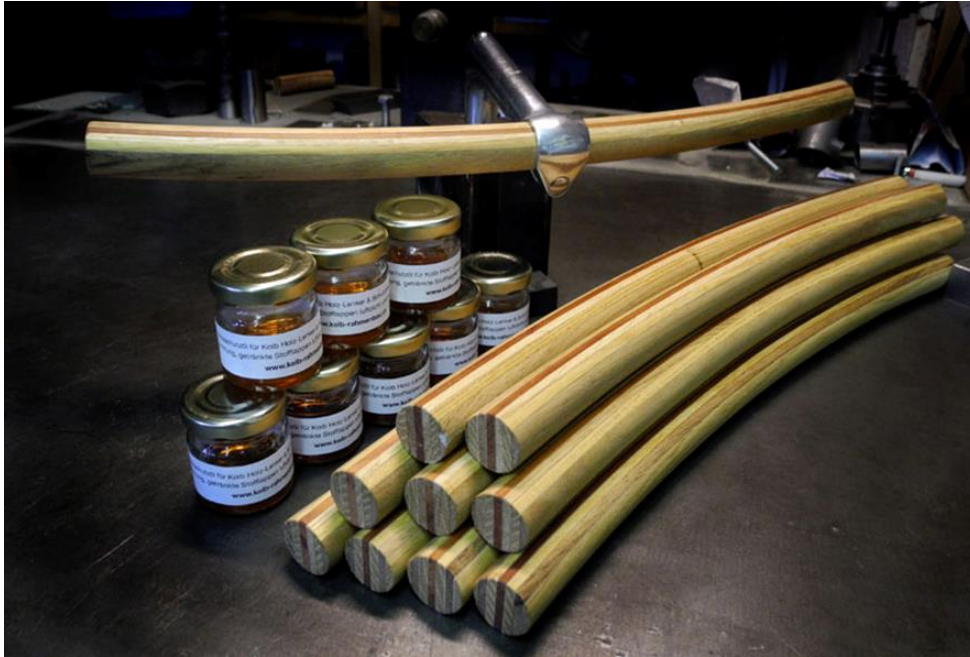
Figure 67. Laminated and curved Wooden Handlebars. Retrieved from https://www.flickr.com/photos/kolb-rahmenbau/6347546756
