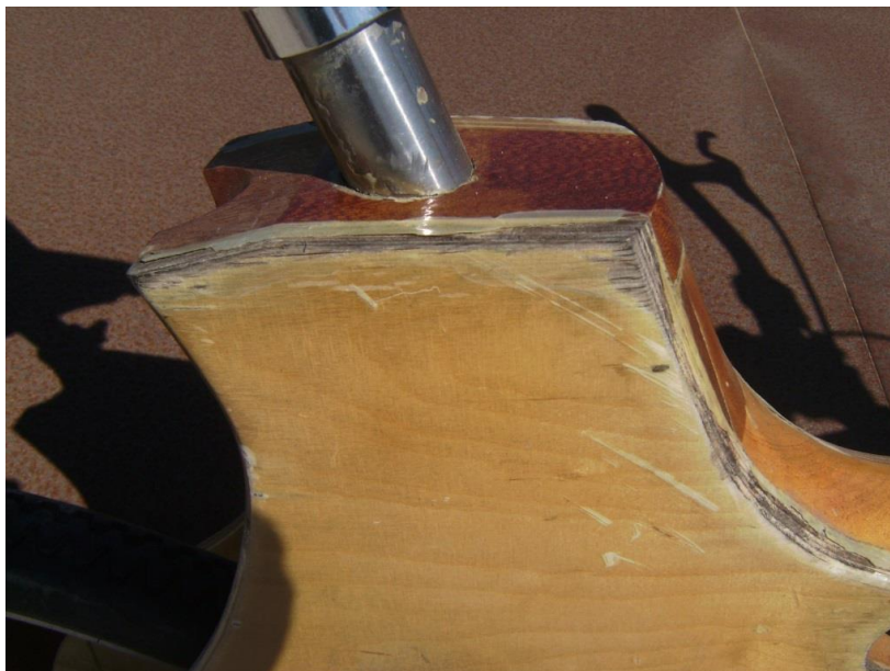
Figure 178. Xylon Hybrid Flaking and Weather Damage. Taylor, Nicholas. 2015
