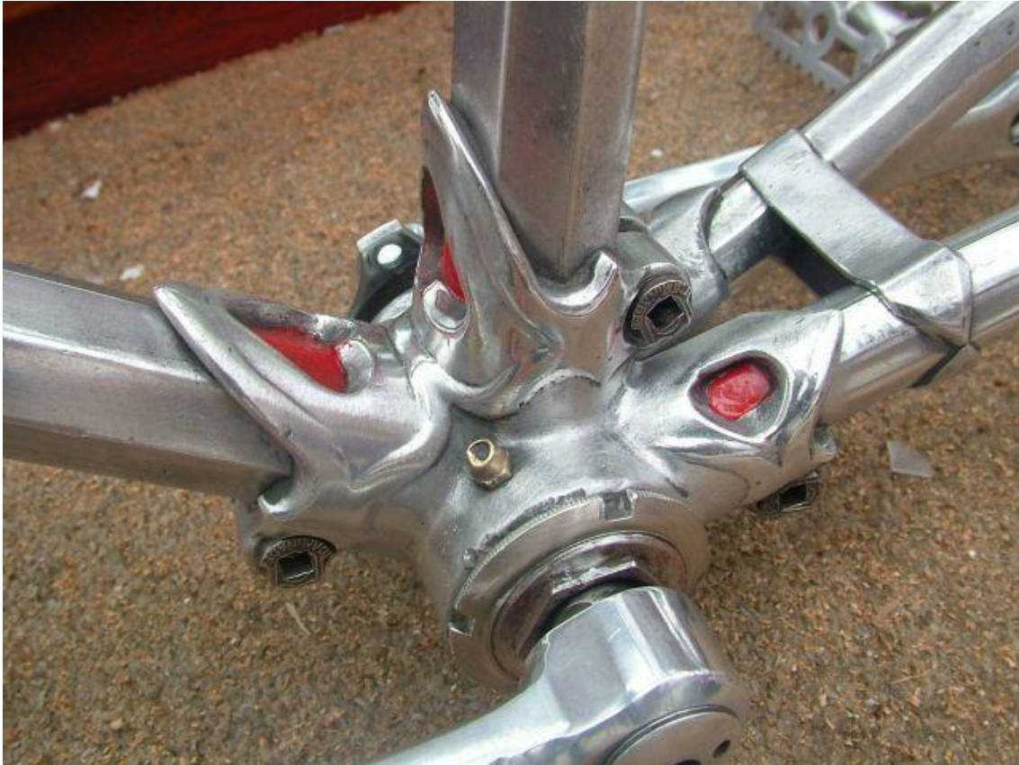
Figure 19. Caminargent Aluminium Bicycle Frame manufactured by Caminade of Paris circa 1937. Retrieved from http://forums.thepaceline.net
