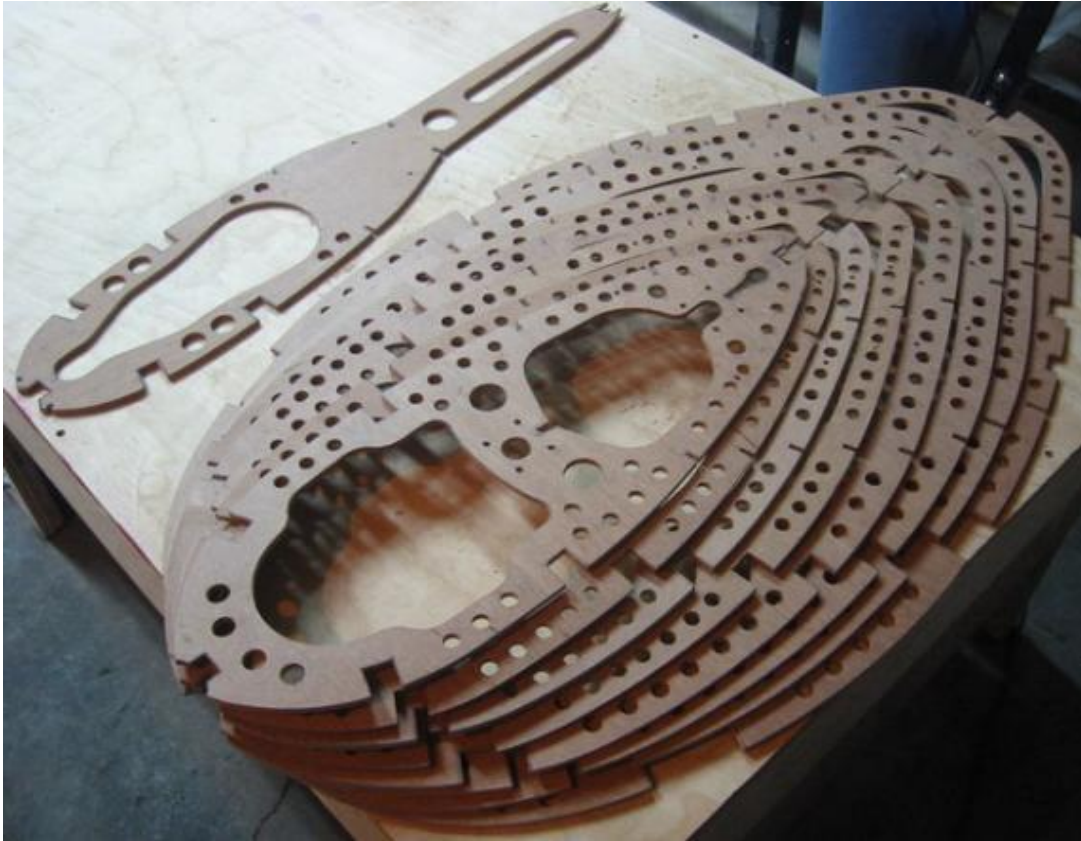
Figure 217. Lightened Plywood Aircraft Bulkheads. Retrieved from http://www.brucespitfire.com/fuselage-page-6.html
