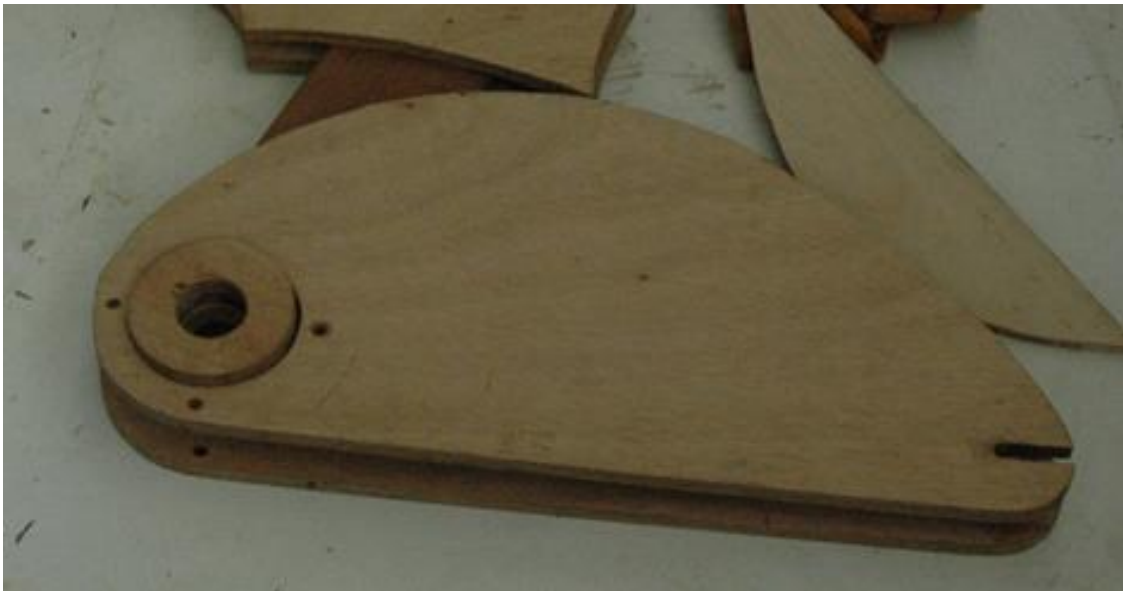
Figure 124. Main Body of Wooden Bicycle Frame Mock-up – Taylor, Nicholas. 2005
