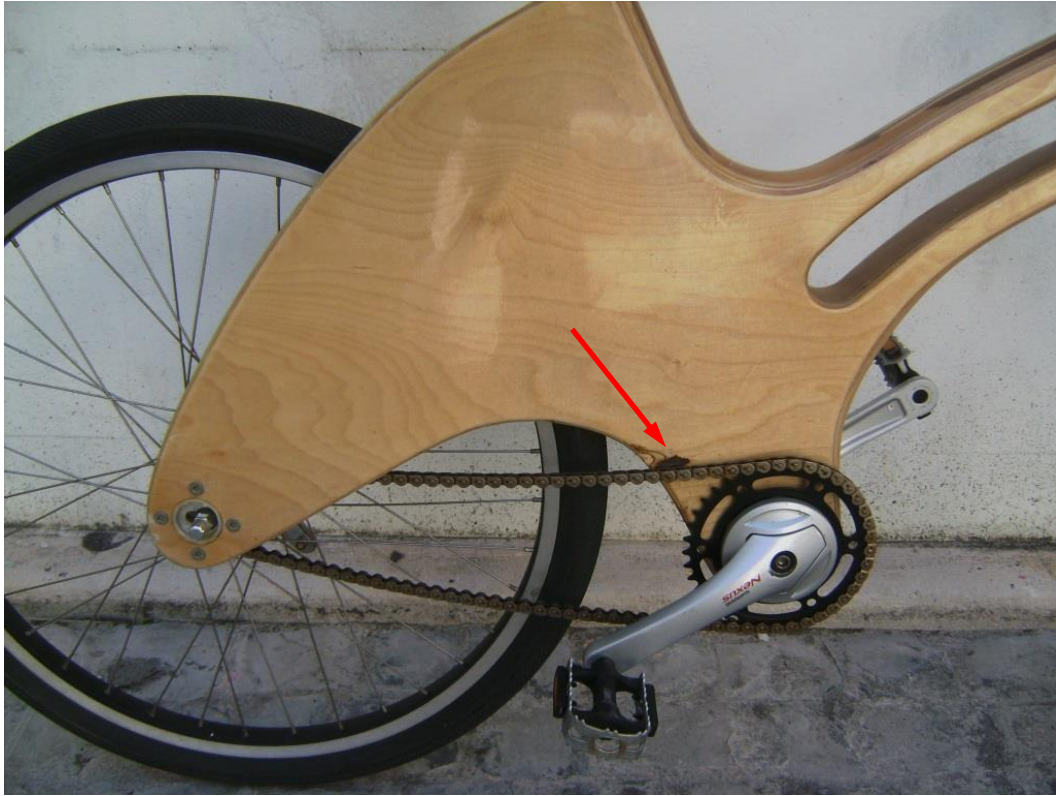
Figure 181. Xylon Klassic exhibits Intact Lacquer but Abrasion to the Frame due to Chain-slap –Taylor, Nicholas. 2015
