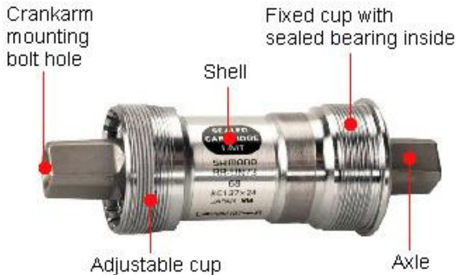
Figure 63. Bottom Bracket Axle Sealed Cartridge. Retrieved from http://www.parktool.com/
