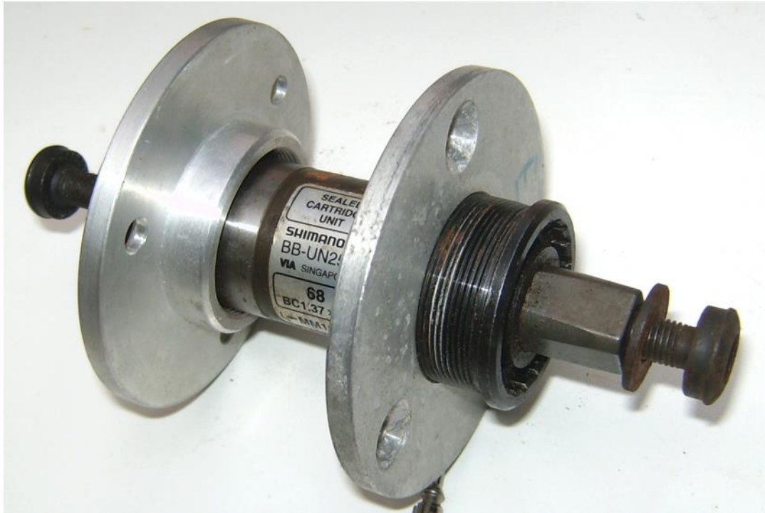
Figure 196. Xylon Two Part Bottom Bracket with Sealed Cartridge Unit in Position –Taylor, Nicholas. 2015
