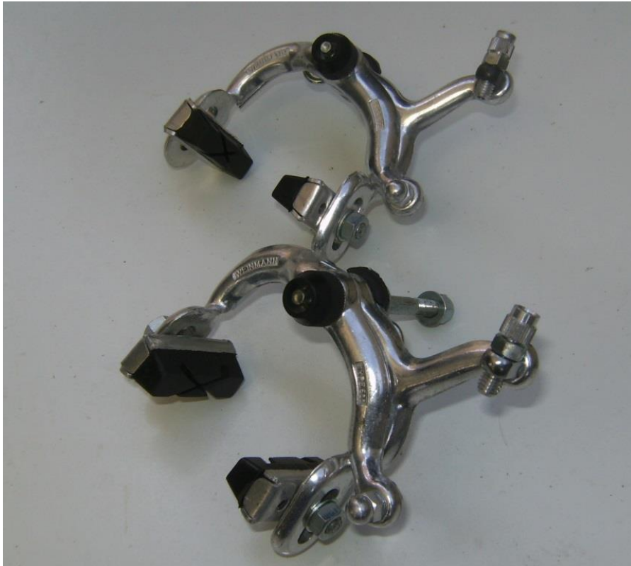
Figure 190. Single Pivot Side Pull Calliper Brakes – Taylor, Nicholas. 2015
