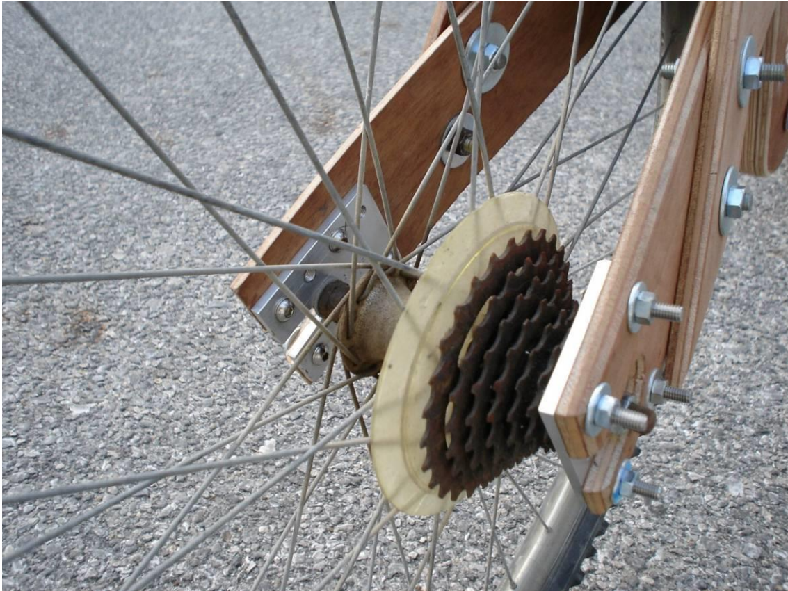
Figure 139. Xylon #1 Initial Trials – Rear Dropouts – Taylor, Nicholas.
