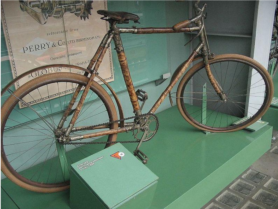
Figure 115. An Original Bamboo Bicycle circa 1895. Retrieved from http://bamboobicycleclub.org/bamboo-bikes-new-concept/
