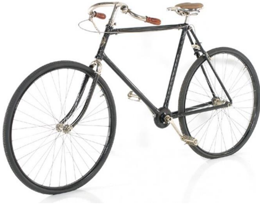
Figure 45. Shaft drive bicycle circa. 1897. Retrieved from https://oldbike.wordpress.com/
