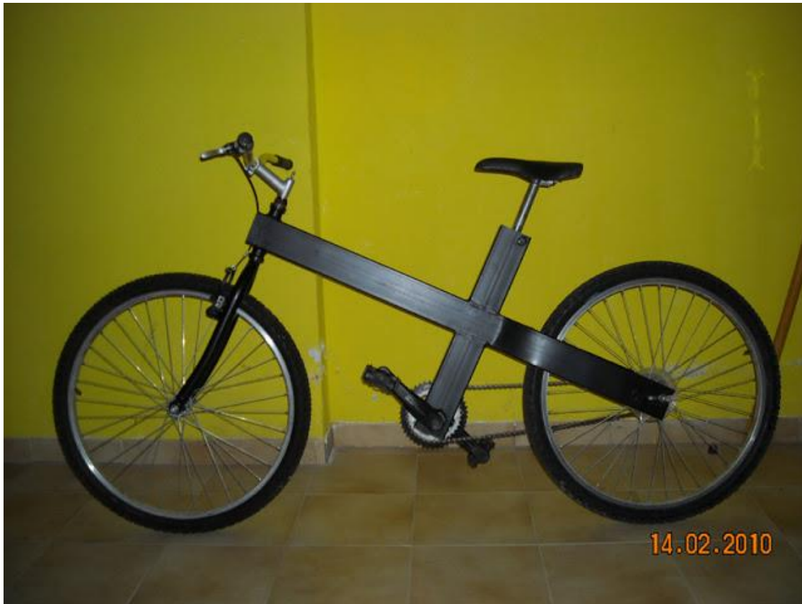
Figure 155. Cross Frame Bicycle Designed by Miguel Garcia 2010. Garcia, Miguel. 2010
