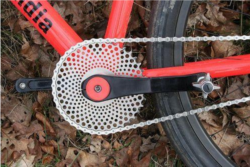
Figure 216. Lightened Chainwheel. Retrieved from http://www.classiclightweights.co.uk/extras/drillium-extras.html
