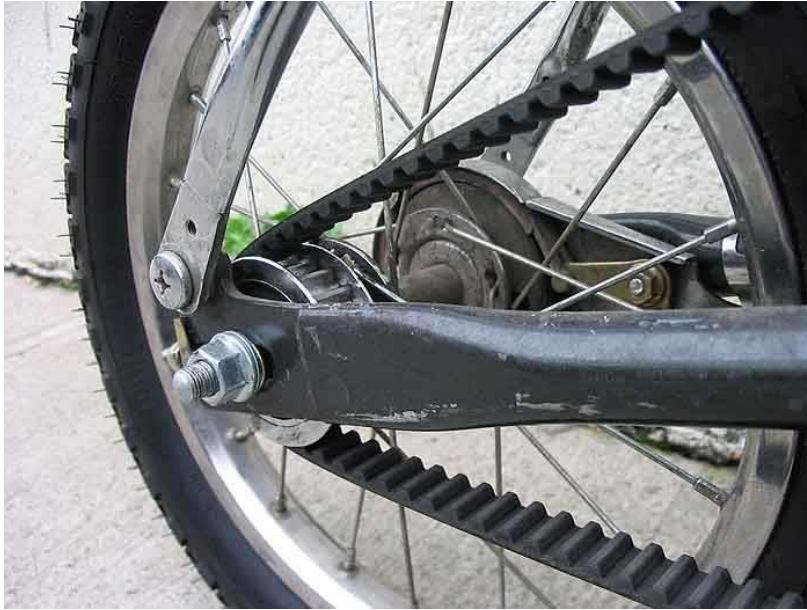
Figure 47. Toothed belt rear hub – Bridgestone Picnica Folding Bike c. 2000. Retrieved from http://bikecult.com/works/archive/04bicycles/picnicaF.html
