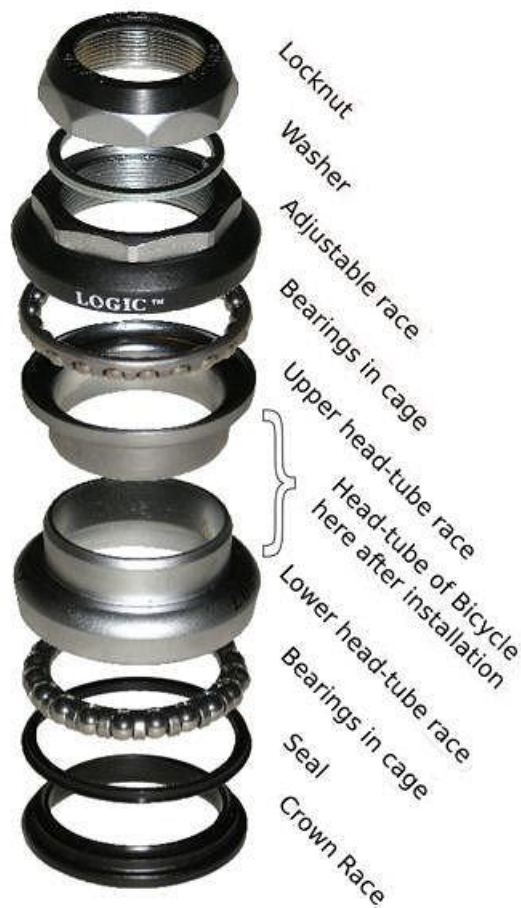
Figure 69. Headset for threaded forks – Sheldon Brown. Retrieved from http://www.sheldonbrown.com/headsets.html
