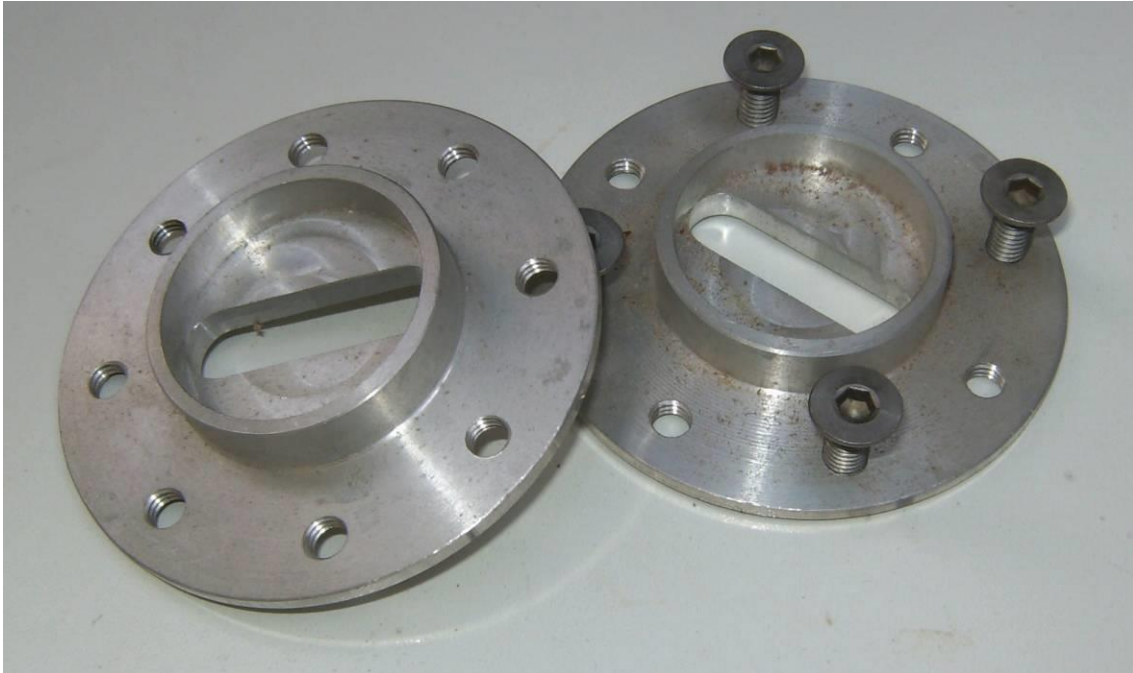
Figure 189. Xylon Turned Aluminium Dropout Prototype #2 –Taylor, Nicholas. 2008
