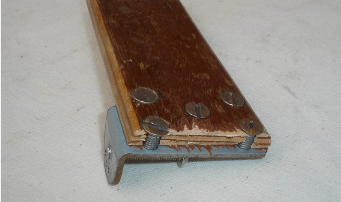
Figure 151. Detail of Failure on Xylon #1 Prototype at V-brake Fixing Holes –Taylor, Nicholas. 2006
