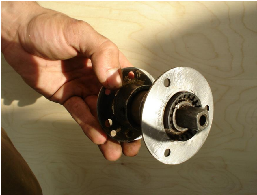
Figure 130. Handmade Two-piece Bottom Bracket Shell Prototype with Flanges – Xylonbikes 2005. Taylor, Nicholas.
