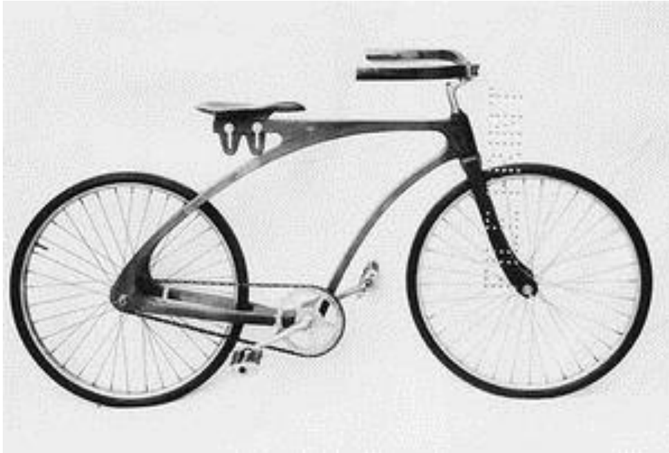
Figure 111. Whalen and Janssen laminated wood frame bicycle. The Smithsonian Collection – Catalog #: 313,040, Accession #: 173,992. Retrieved from http://amhistory.si.edu/onthemove/collection/object_312.html
