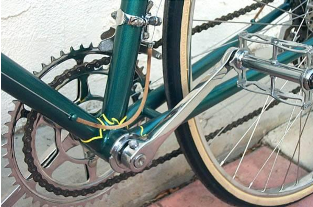
Figure 60. Cottered cranks on a 1970s bicycle. Retrieved from oldtenspeedgallery.com
