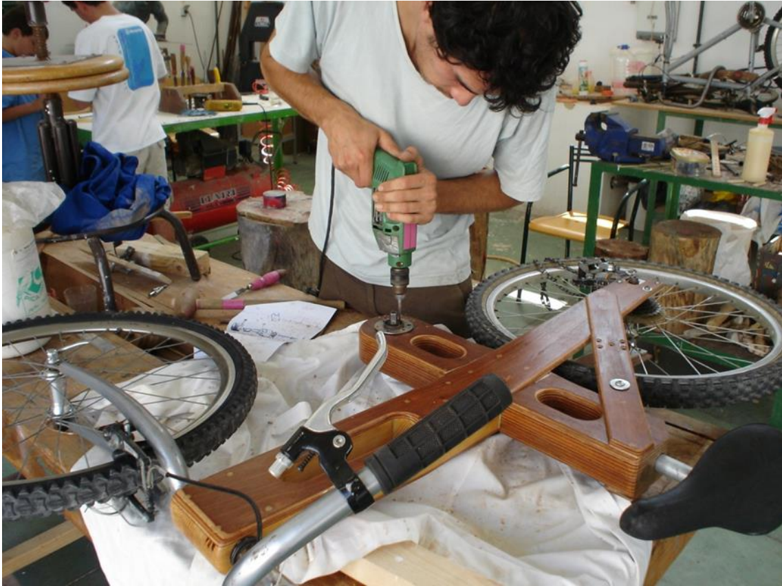
Figure 145. Leonel Mateus Drilling Xylon #1 Frame for Bottom Bracket Fitting –Taylor, Nicholas.
