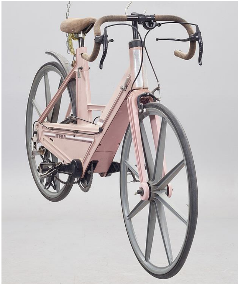
Figure 51. Itera Plastic Bicycle Fitted with Conventional Dropped Handlebars. Retrieved from http://twwhlspls.com/itera/
