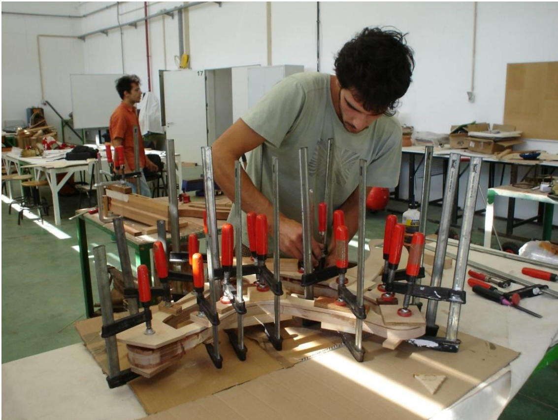
Figure 169. Leonel Mateus Gluing and Cramping the Synergy frame. Taylor, Nicholas. 2005
