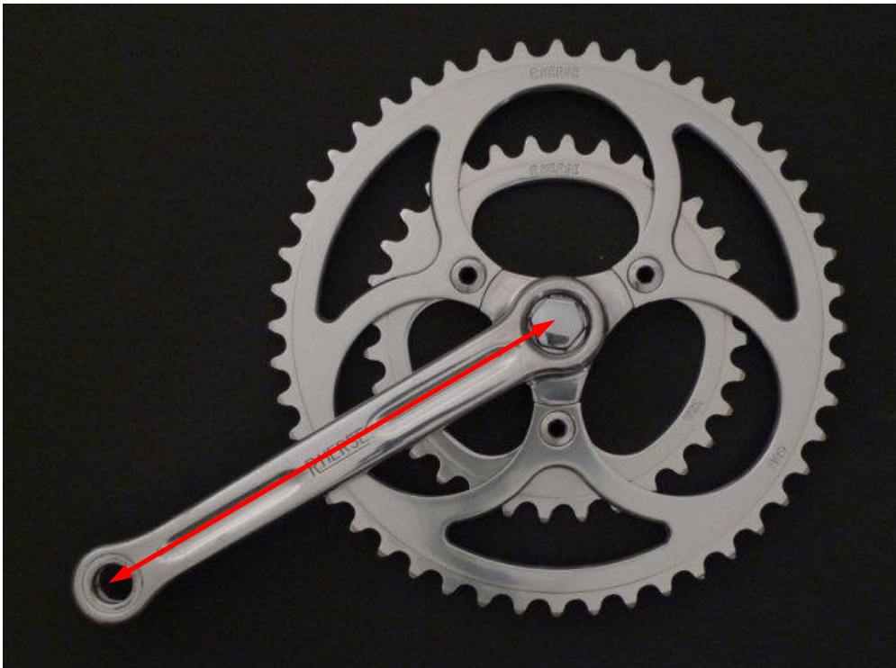
Figure 125. Rene Herse Crankset showing Crank Arm Length. Retrieved from http://velosniper.blogspot.pt/2008/10/wednesday-price-porn-rene-herse-cranks.html
