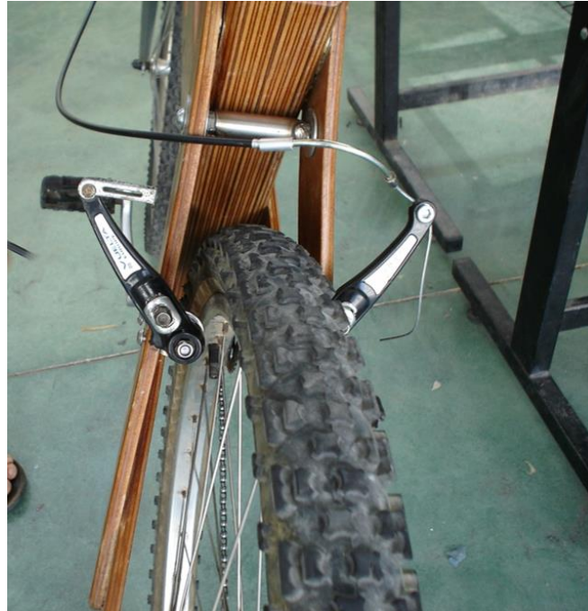
Figure 150. Initial Fitting of V-Brakes on Xylon #1 Prototype –Taylor, Nicholas 2005
