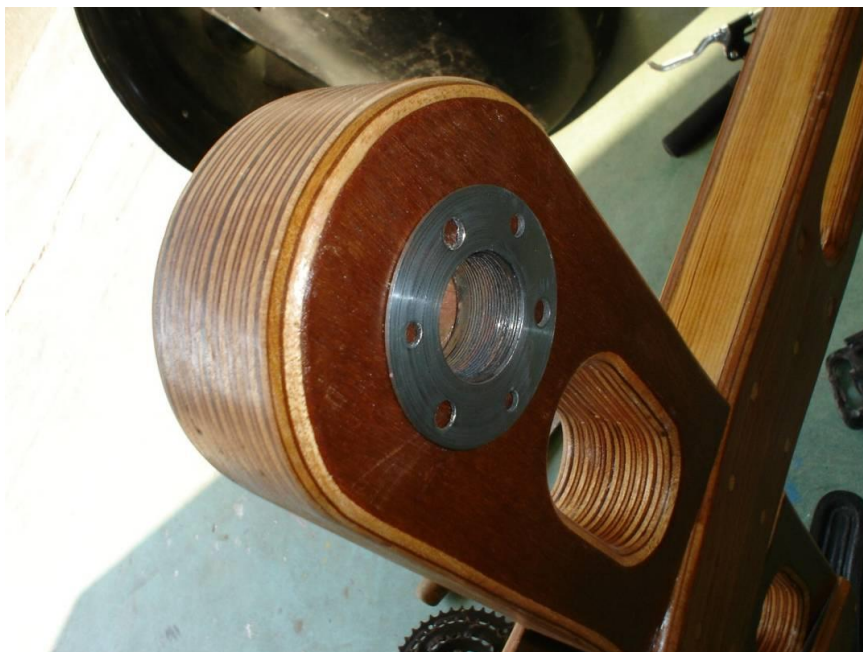
Figure 131. Handmade Two-piece Bottom Bracket Shell with Flanges Trial Fitting to Xylon #1 – Xylonbikes 2005. Taylor, Nicholas.
