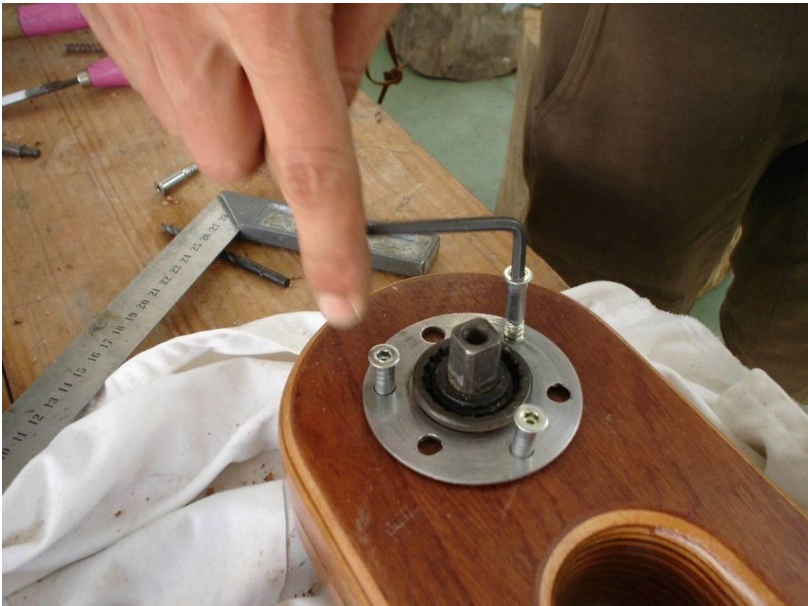
Figure 132. Handmade Two-piece Bottom Bracket Shell with Flanges Trial Fitting to Xylon #1 – Xylonbikes 2005. Taylor, Nicholas.
