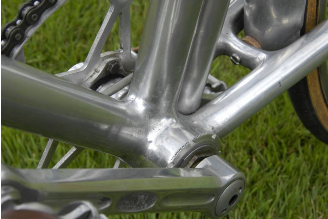
Figure 20. Welded and fettled aluminium bicycle frame by Nicola Barra bicycle built for Garin cycles in 1941. Retrieved from https://vintagebicycle.wordpress.com/2011
