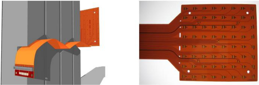
Figure 1. Left: Drawing of the Dice-Board, with the pigtail passing through the copper shield. Right: Picture of the kapton Dice-Board.
